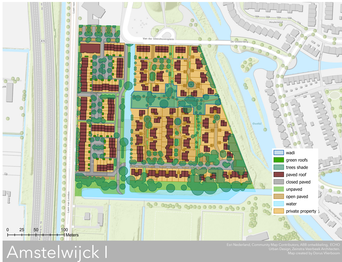
Figure 4.1: Climate-adaptive measures applied in Amstelveen I
