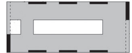
Short wall in x direction as collector members would effectively resist the inertial force.
