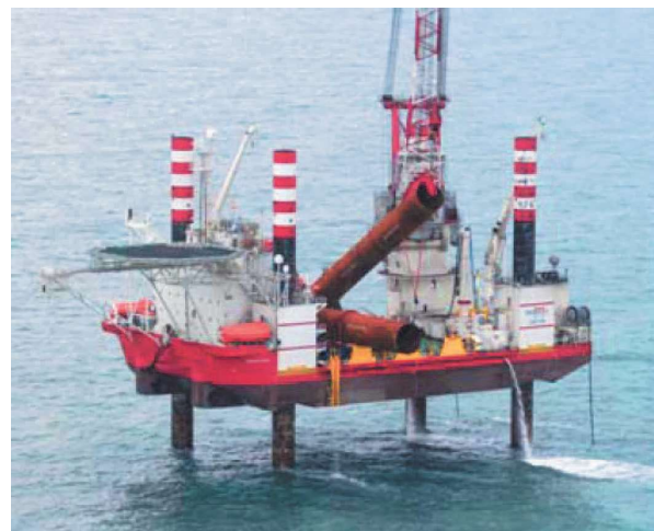
Figure 1-2: Jack-up ship the SeaJack's Zaratan (source: HeavyliftSpecialist.com )
