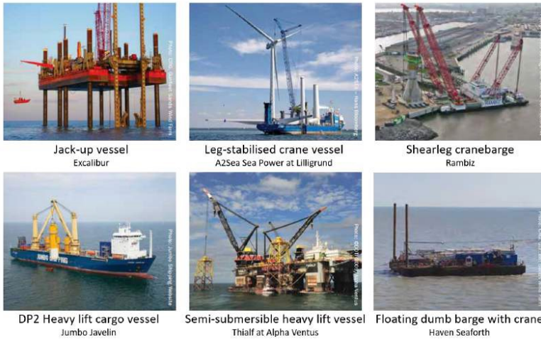
Figure 1.4: OWT installation vessels
