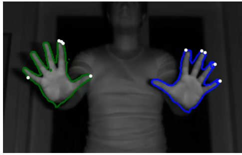
(a) Time-of-Flight (TOF) based finger tracking using Microsoft Kinect V2 camera [21]
