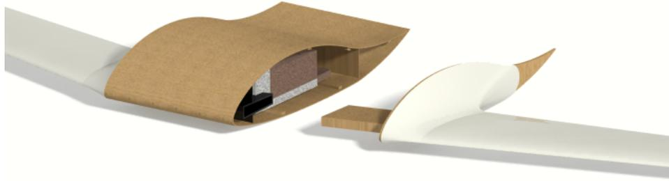
**Figure 7.10:** Render of the internal structure of the glider. The white boxes indicate the crash structure, the brown box represents the payload.
