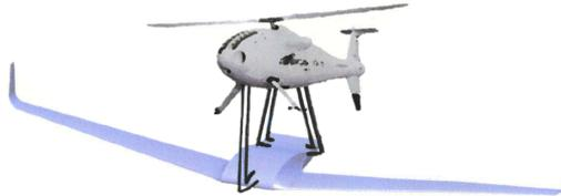
Figure 6.27: Rigid launch attachment; chosen design.
