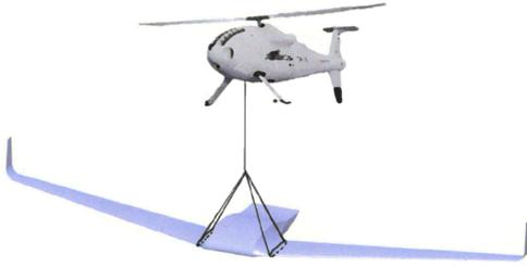
Figure 6.25: Launch attachment with simple rope.
