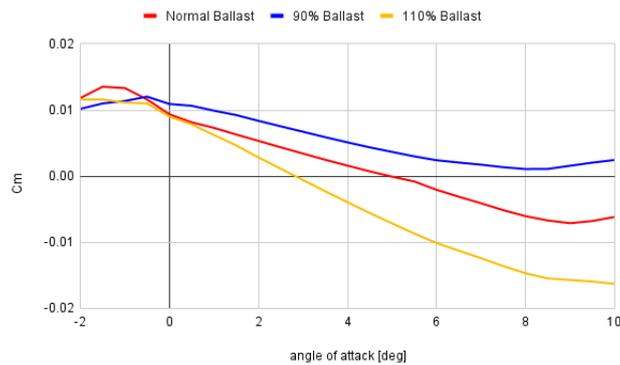
**Figure 5.26:** Comparison of the stability of the different ballast masses
