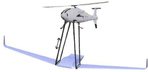
Figure 6.26: Launch attachment with moving rigid rod.
