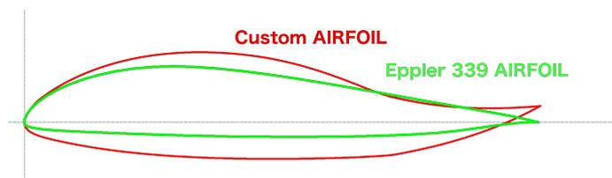
Figure 5.10: Difference between the Eppler 339 and the custom reflexed airfoil
