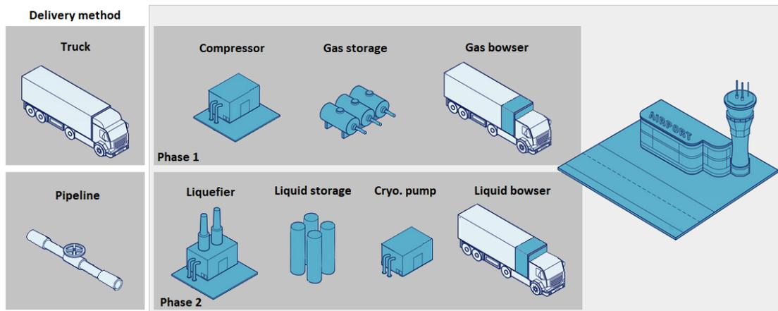
Figure 5: First and second phases of transition represented in two streams (flow direction left to right) one delivering gas and the other delivering liquid hydrogen to aircraft (elements in this image were obtained from Airbus S.A.S., 2021).
