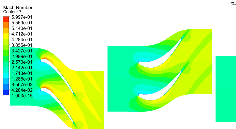
Figure 3.44: Mach contour of the shrouded turbine case at the mean radius.
