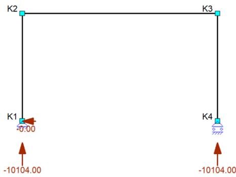
Figure 7-25 - Foundation forces method 3a
