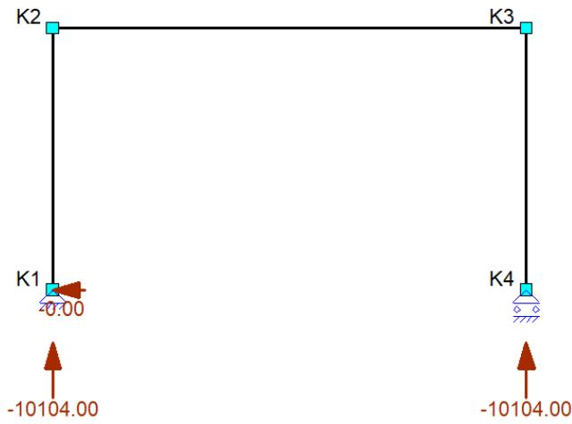
Figure 7-19 - Forces on foundation portal crane
