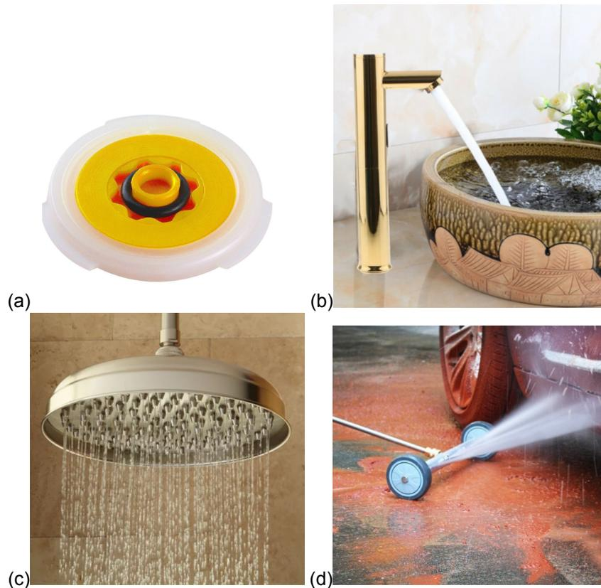
Figure 8.2: Examined watersaving equipment used for the designs. In the design, flowregulators (a) that guarantee a constant, predefined flow rate can be implemented in the taps inside the restaurant. Furthermore, the design contains sensor taps (b) in the toilet, an efficient shower head (c) and an efficient water broom (d) that can be used for cleaning activities.
