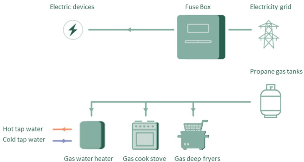
Figure 12.5: Schematic representation of the current energy infrastructure of Irmão
