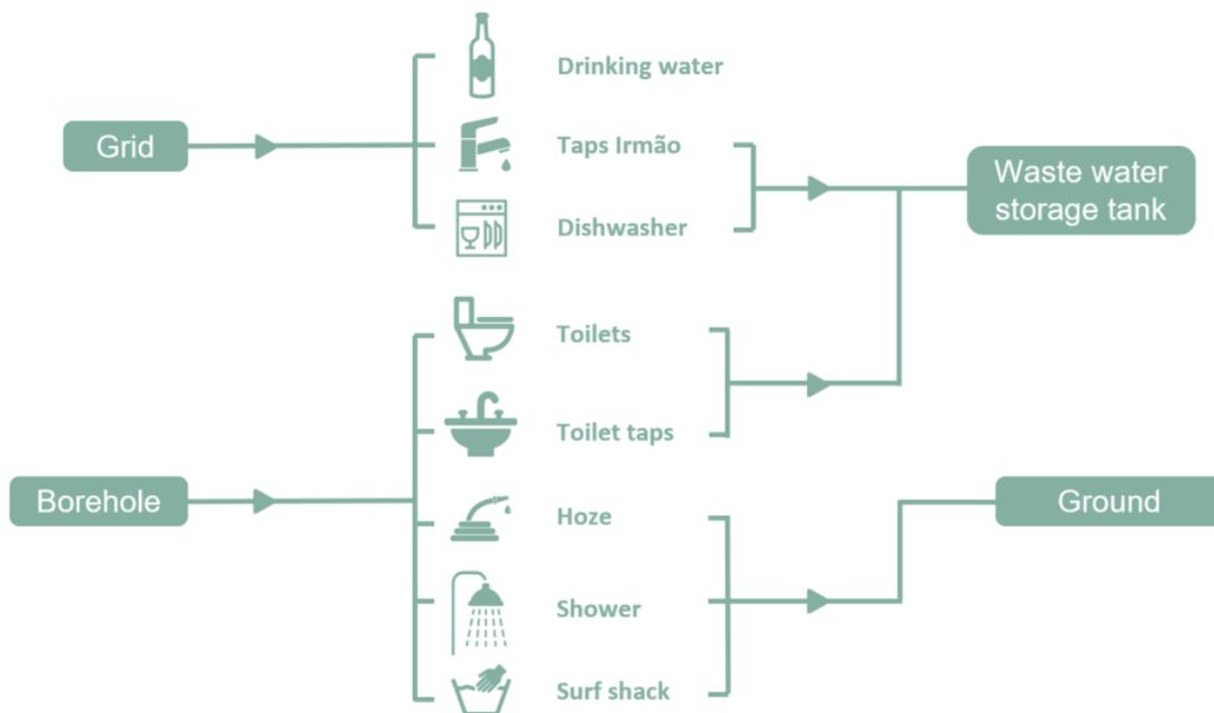
Figure 6.2: Systematic display of the current water infrastructure.
