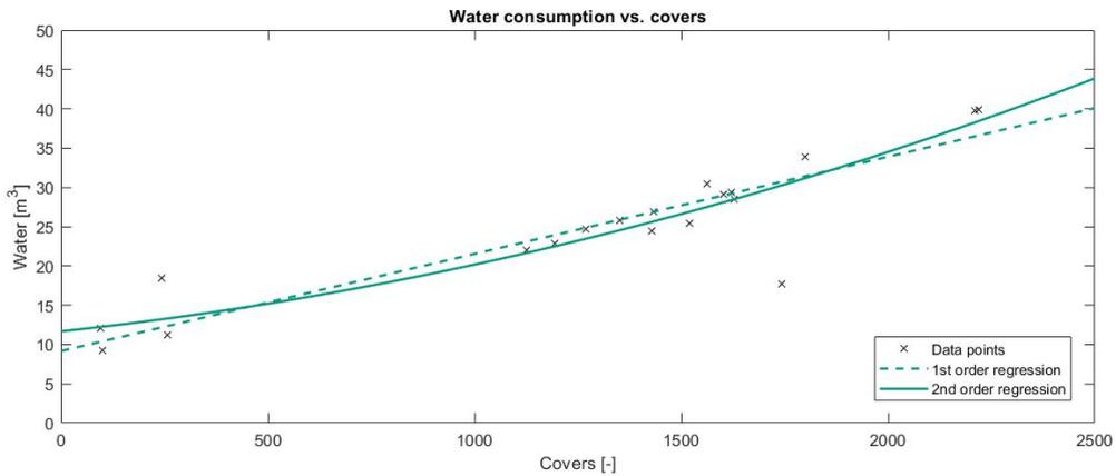
Figure 6.4: Result of second order polynomial regression between number of monitored weekly covers and the weekly amount of water obtained from the grid.
