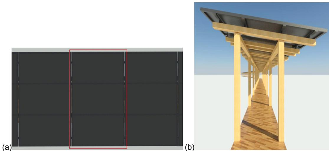
Figure 14.15: (a) Top view of the solar path with in red indicated a single solar path unit. (b) Front view of the solar path seen from the restaurant, made in Revit.
