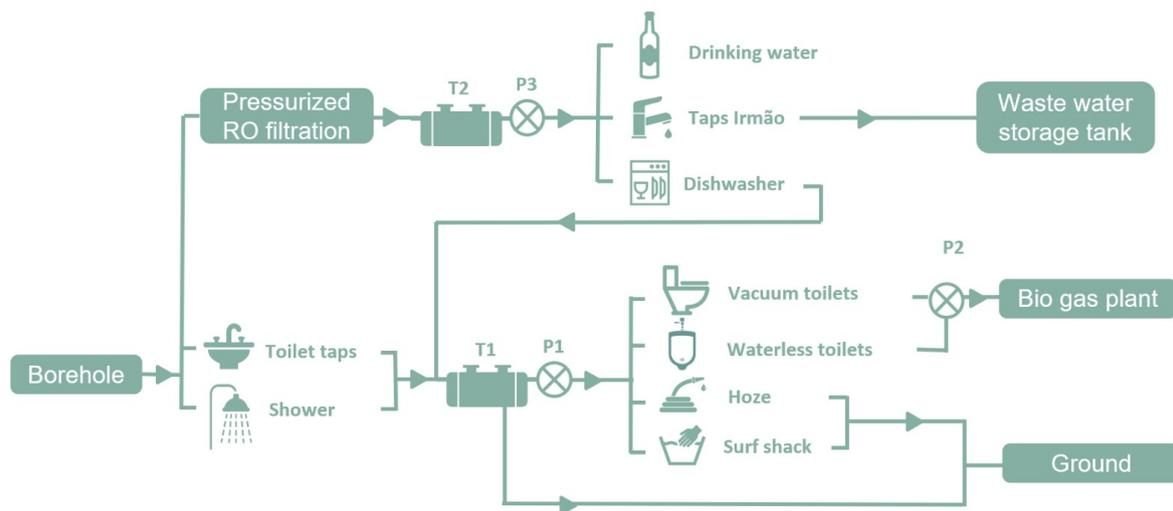
Figure 8.4: Systematic display of infrastructure proposal in which the system can be build form scratch, i.e. the future beach pavilion.
