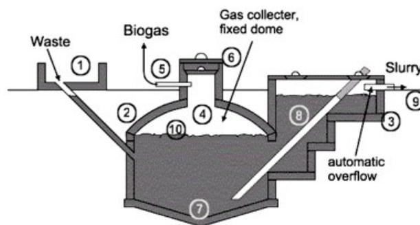
Figure 11.2: Fixed dome biogas plant (Radtke, 2016)
