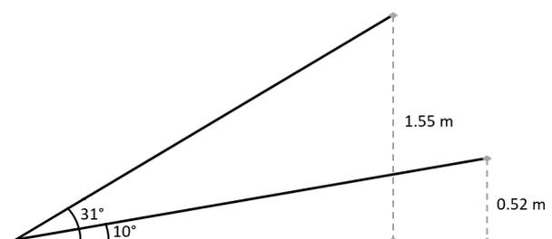
Figure 14.16: Schematic representation of the difference in height of the solar path dependent on the tilt angles of the solar panels.
