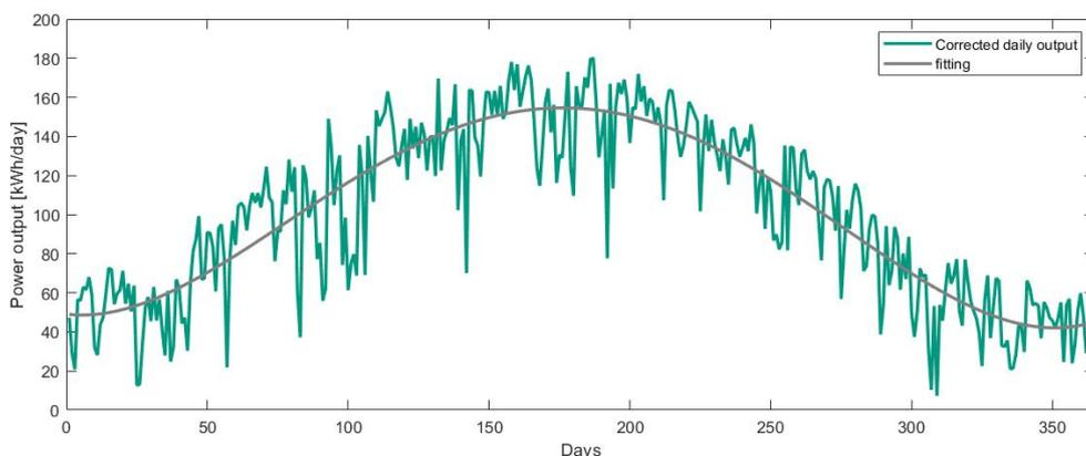
Figure 15.2: Power output of the rooftop PV solar system
