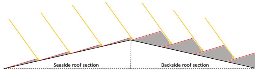
Figure 14.13: Schematic representation of the tilted panels on the seaside and backside roof section with irradiance coming from the sun at a Sun height of 60 degrees
