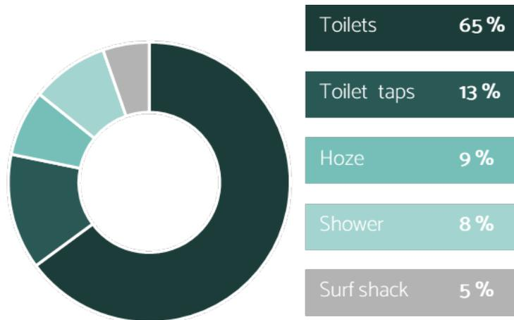
Figure 6.7: Water consumption ratio between the devices connected to the borehole.
