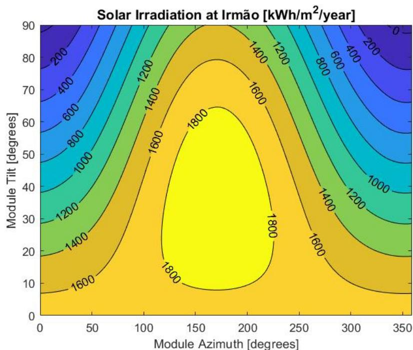
Figure 14.8: Irradiance per tilt and azimuth angle at Irmão. Graph created with Matlab
