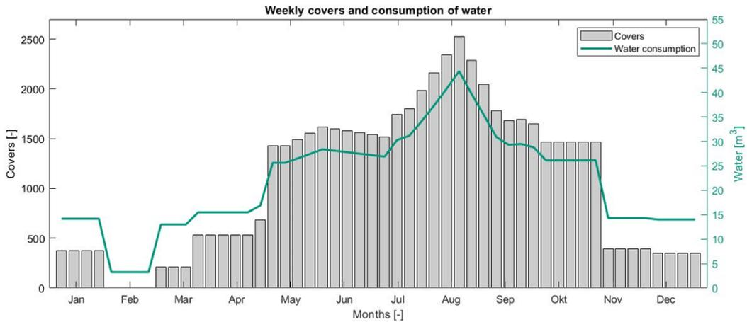
Figure 6.5: Weekly water consumption from water grid estimate, based on results of second order polynomial regression between monitored weekly number of covers and weekly amount of water obtained from the grid.
