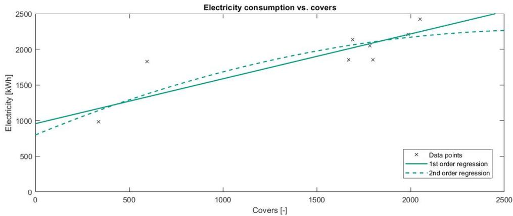
Figure 12.7: First and second order regression of the covers versus electricity consumption based on invoices and measurements
