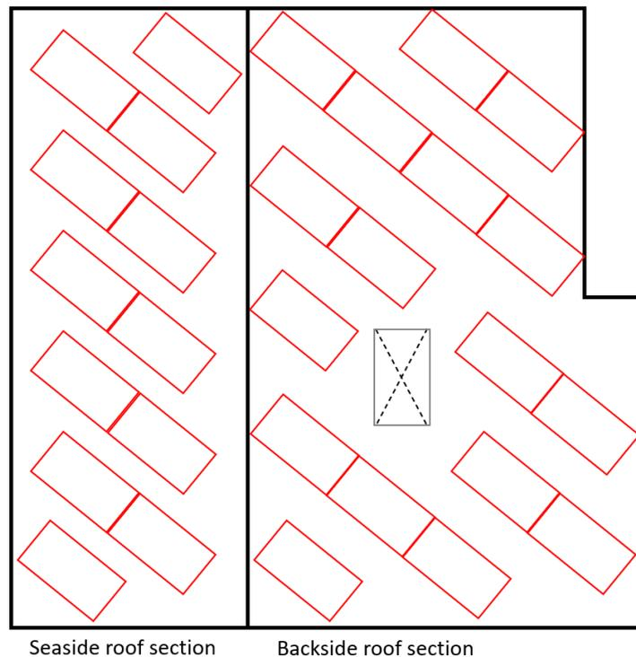
Figure 14.14: Schematic top view representation of the ideal tilt configuration
