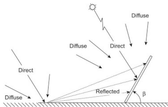
Figure 14.5: Schematic representation of the 3 components (Reca-Cardaña and López-Luque, 2018).
