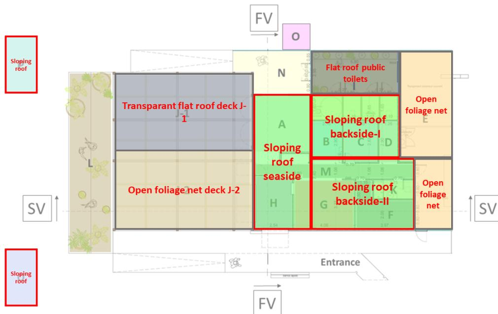
Figure 3.4: Blueprint of the top view of Irmão with the corresponding roof sections.
