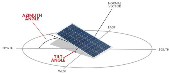
Figure 14.7: Azimuth angle and tilt angle (Electrical, 2019)
