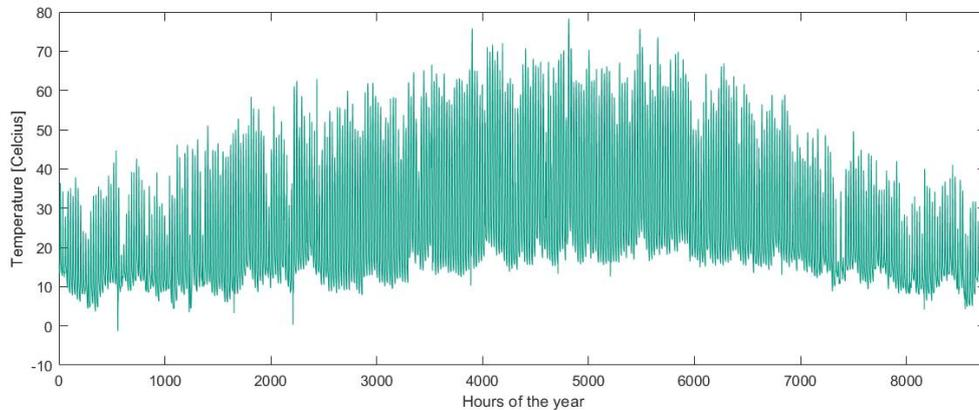
Figure 14.9: Temperature of the PV panels during the year
