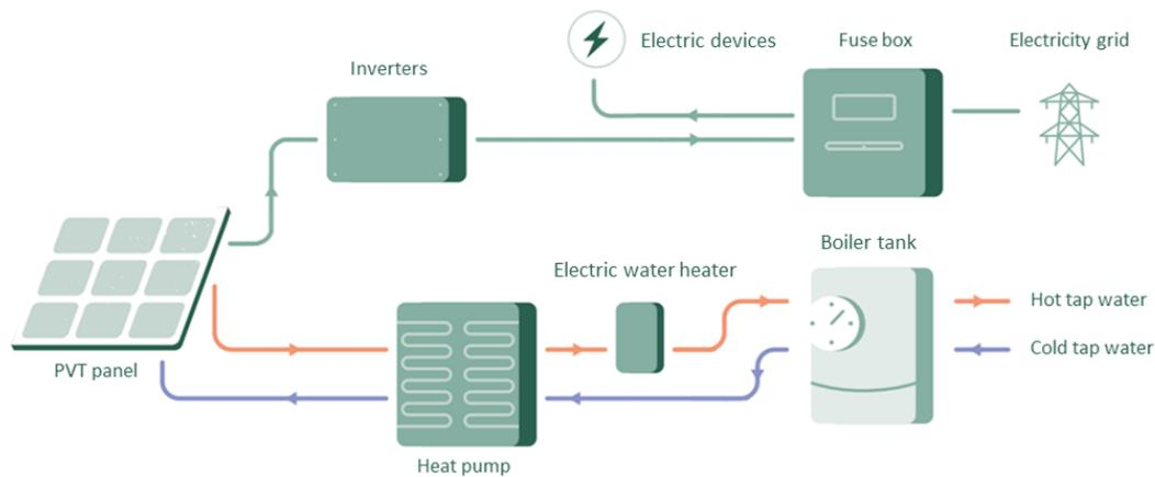
Figure 14.3: Total PVT system configuration.
