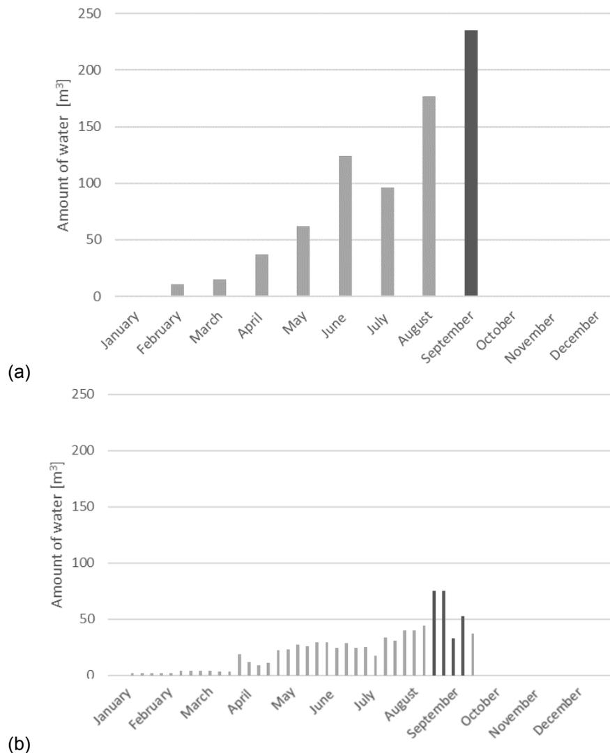
Figure 6.3: Data of monthly water consumption from public water grid (a), obtained from the owner in the form of monthly water bills. The monthly data has been translated into weekly data (b), this is done to be able to analyse peak consumption. The bars having a darker colour present the month in which the pump of borehole was not working and therefore gives a distorted result.
