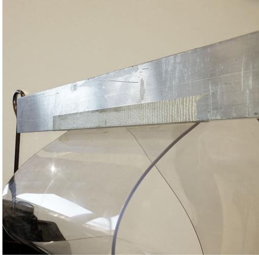
Figure 13: Knife-edge bearing for the application of a vertical motion along a line of the surface. Double-sided adhesive tape holds the corner of the aluminum bar on its place.
