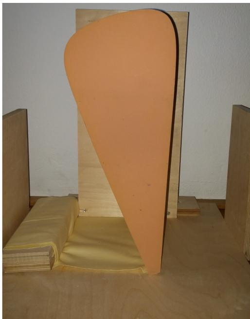
Figure 9: One sided mould out of high-density foam material.
