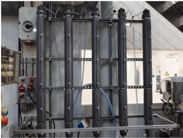
Fig. 3. Laboratory scale Denutritor® columns. (Source: Author).
