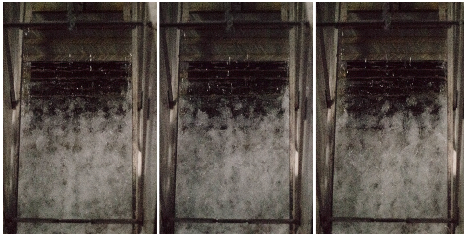
Fig. 18. High-shutter speed top view photographs of skimming flow on the 45° stepped chute – Main flow direction from top to bottom, d_c/h = 1.2 , Re = 5.2 \times 10^5 , \theta = 45^\circ , h = 0.10 m, \lambda/k = 2.0 , 24 MPixels dSLR photographs, Shutter speed: 1/8000 s, with 120 ms between photographs (from left to right).
