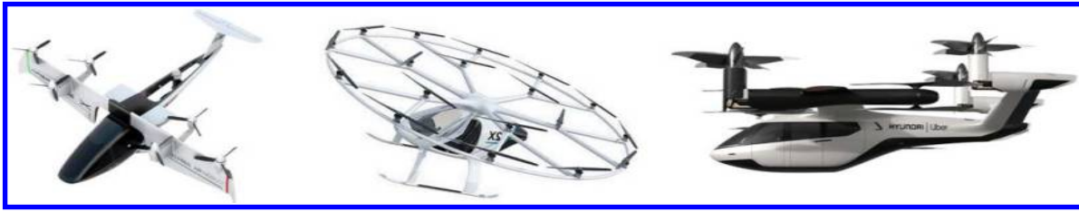
Figure 1. Various eVTOL vehicles that have been under development in recent years. Many of the advanced air mobility concepts include open rotor propulsion technologies; a wide variety of multi-rotor layouts exists among different designs. Photo credits from left-to-right: AirSpaceX, Volocopter and Hyundai/Uber.
