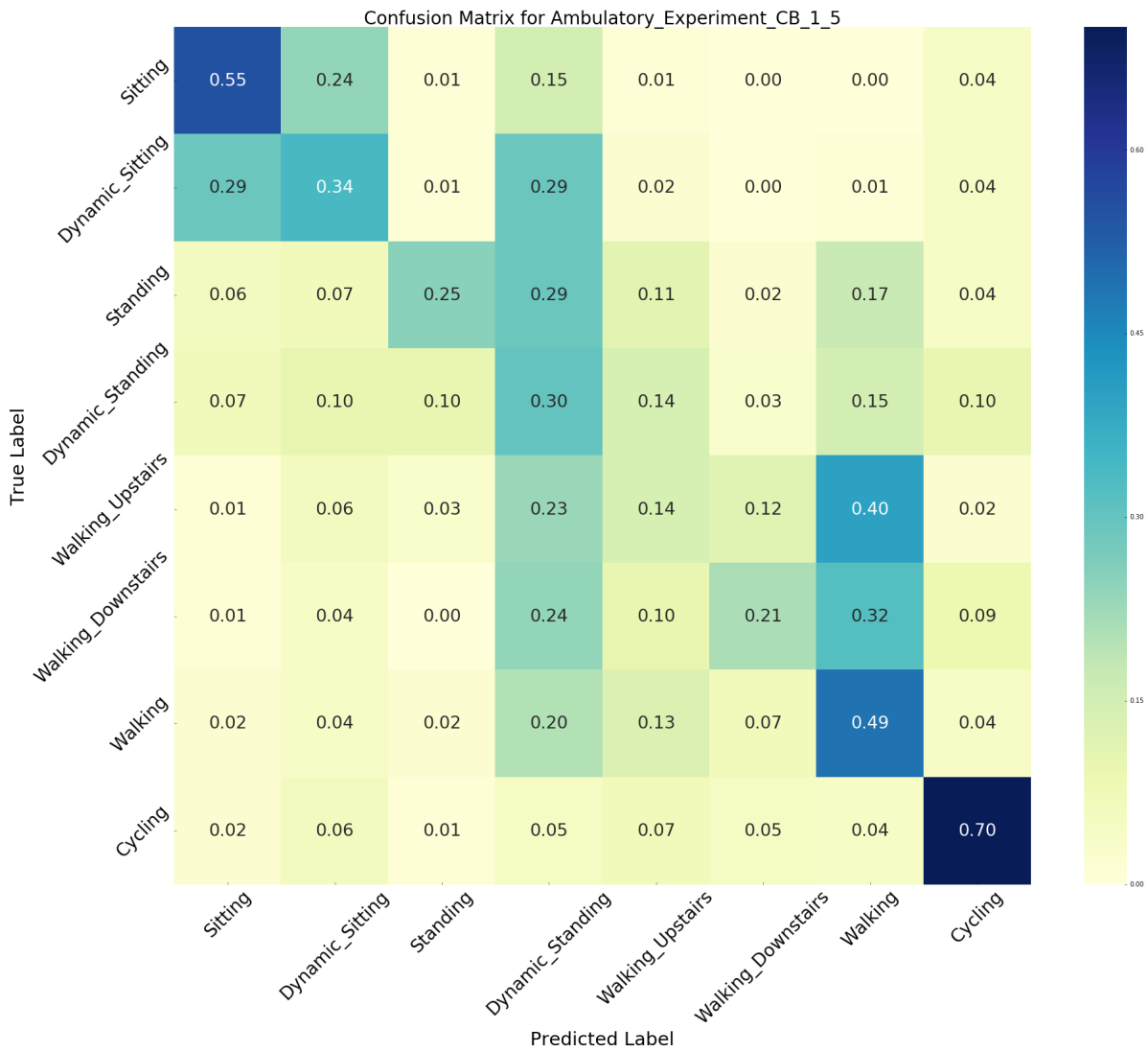
Figure 5.17: The confusion matrix for the chillband (CB) sensor is presented. The training set consists of 40 subjects from the Controlled Study, while the test set consists of 22 subjects from the Free-Living Study. The validation is for the Free-Living Study, by detecting 8 activities.
