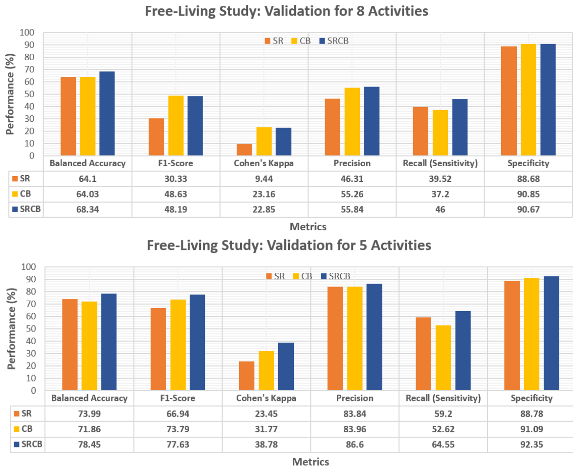
Figure 5.14: The validation model B is evaluated for predicting 8 activities (top graph) and 5 activities (bottom graph) through different metrics. The training set consists of 40 subjects from the Controlled Study, while the test set consists of 22 subjects from the Free-Living Study. SR dataset represents the stingray sensor, CB dataset represents the chillband sensor, and SRCB dataset represents the combination of stingray and chillband sensors.
