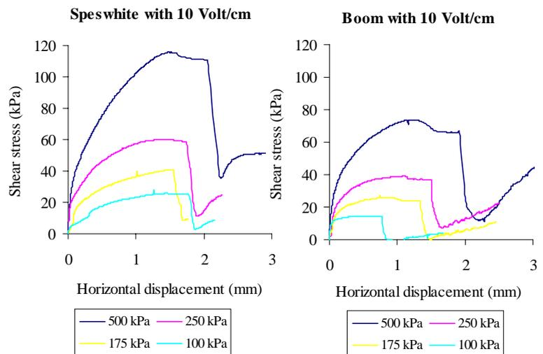
Figure 8 : Effect of normal stress for (left) Speswhite and (right) Boom clay using a potential gradient 10 Volt/cm.
