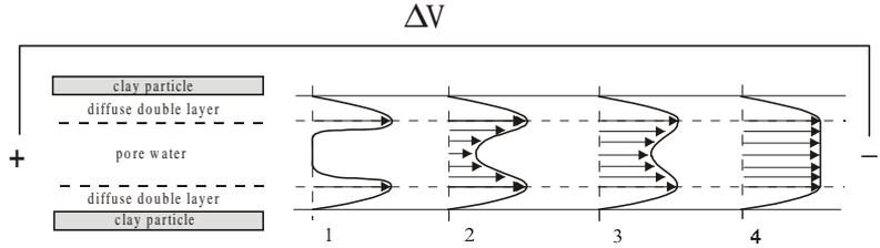
Figure 1 : Development of electro-osmotic flow between two clay particles, with arrows representing flow velocities. 1) switching on of electric field, 2)-3) development of electro-osmotic flow, 4) steady-state flow (after Tikhomolova, 1993).
