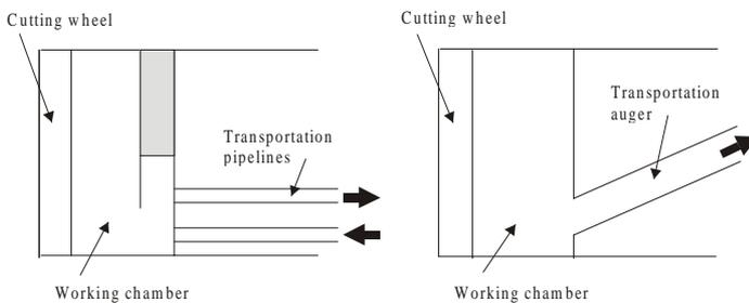
Figure 9 : Locations where adherence can occur. **Left:** at a slurry shield machine **Right:** at an EPB shield machine
