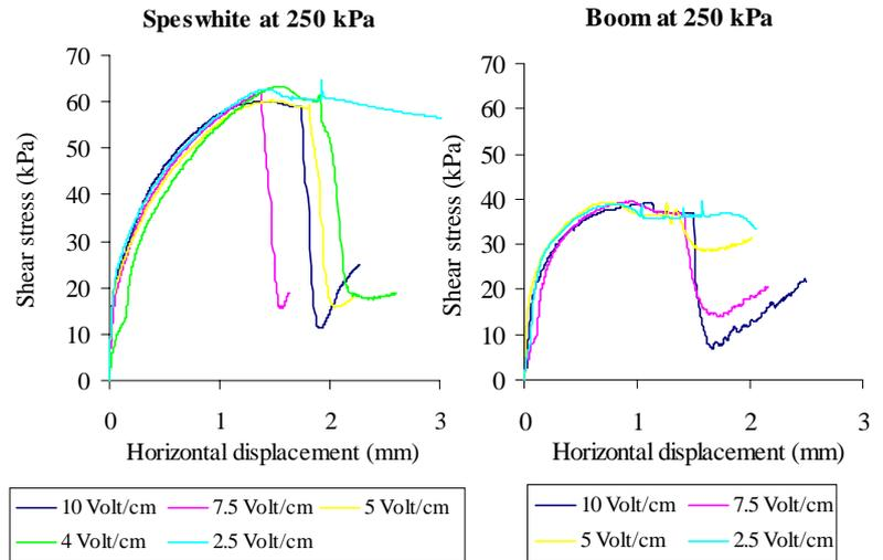
Figure 6 : Effect of the potential gradient for (left) Speswhite and (right) Boom clay at a normal stress of 250 kPa.
