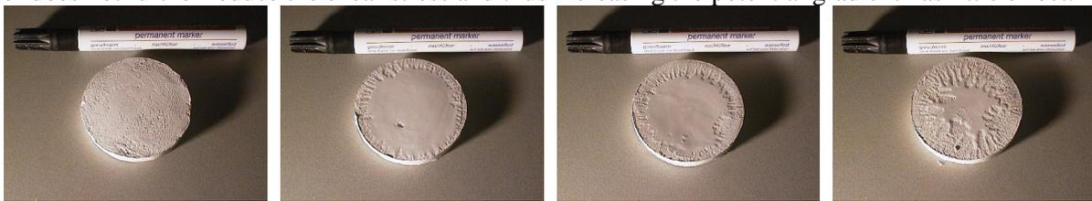
Figure 7 : Picture of contact surface of samples using from left to right: 2.5, 5, 7.5, and 10 Volt/cm.
