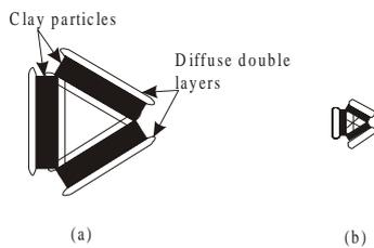
Figure 2 : A model (not to scale) of a cross-section of the pore space in relation to the diffuse double layers. **a:** Three large kaolinite clay particles. **b:** Three small illite particles. (after Shang, Lo and Quigley, 1994)
