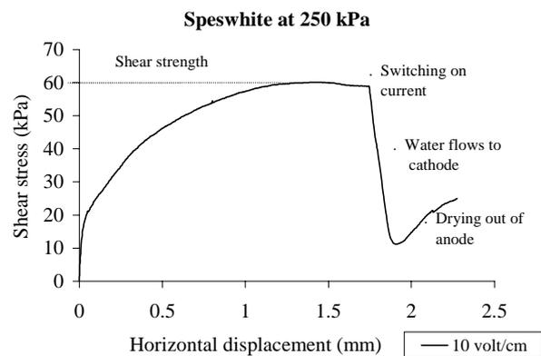
Figure 4 : Effect of electro-osmosis on the shear stress of Speswhite clay at 250 kPa normal stress using a potential gradient of 10 Volt/cm.
