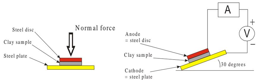
Figure 3 : Tilted-plate test. **Left:** a force is applied to the sample. **Right:** the plate is tilted and an electric current is applied.
