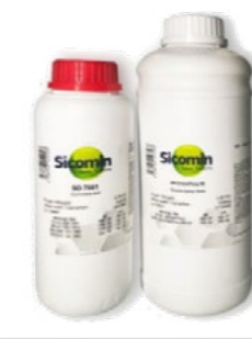
Figure 26. Bio-Epoxy Used in fabrication
