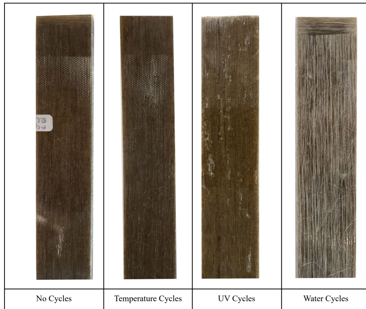
Figure 36: Panel F4 before and after weathering conditions
