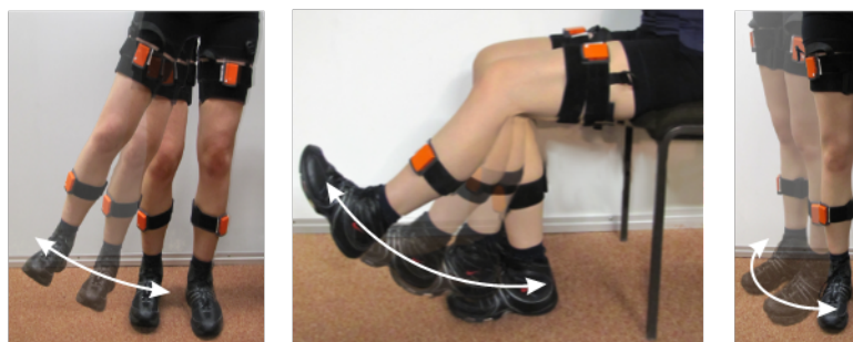
Figure 2-12 Calibration motions to determine orientation of IMU regarding to body segment (Seel, Raisch et al. 2014)
