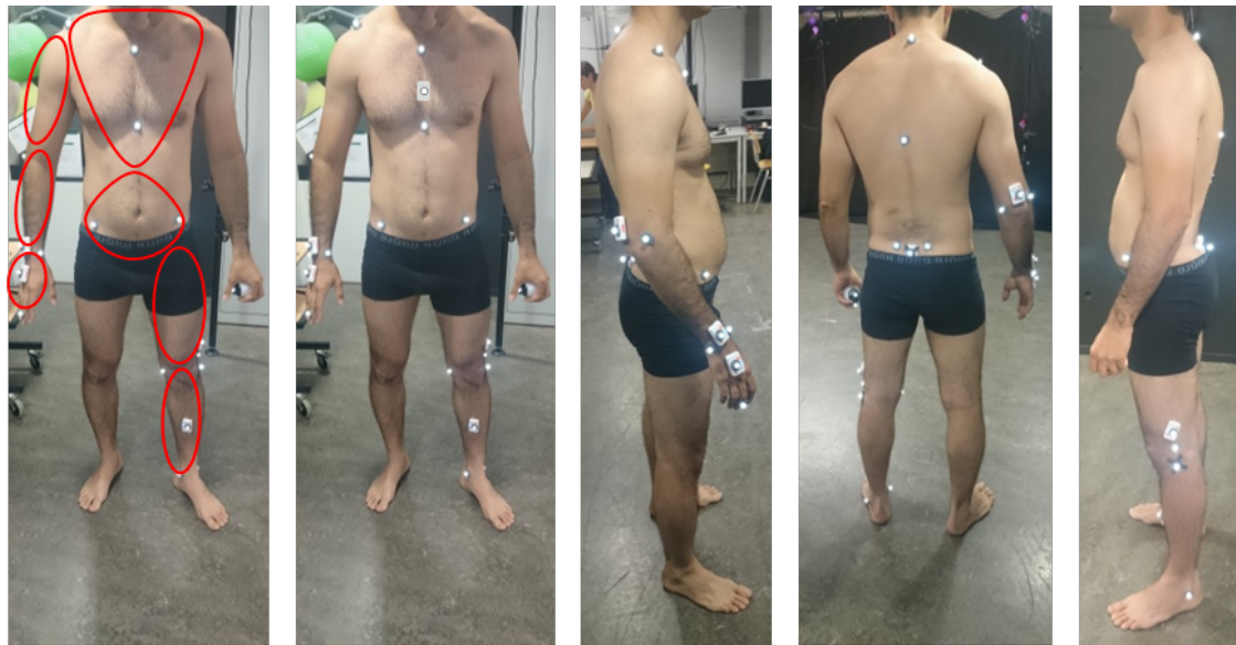
Figure 3-6- Markers and IMU placement; subject is equipped with markers and IMU sensors, identifying 7 body segments.
