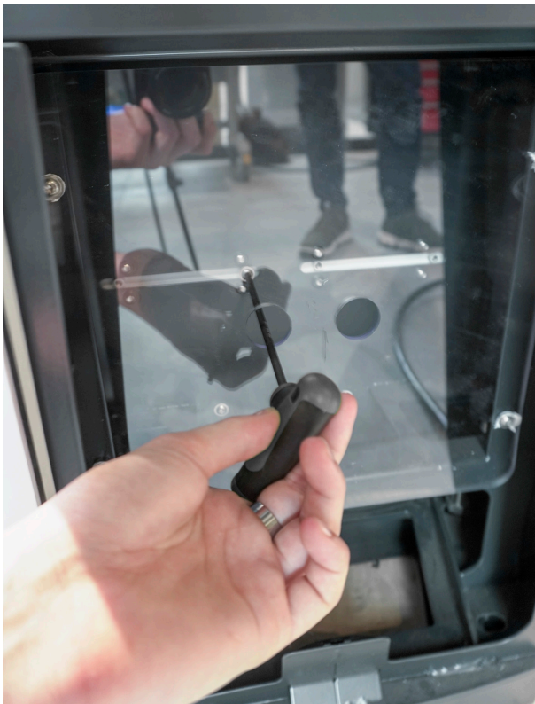
Figure 26. To remove the side panels 4 screws have to be removed with a Torx 25 screwdriver, a penalty for low visibility is given here.
