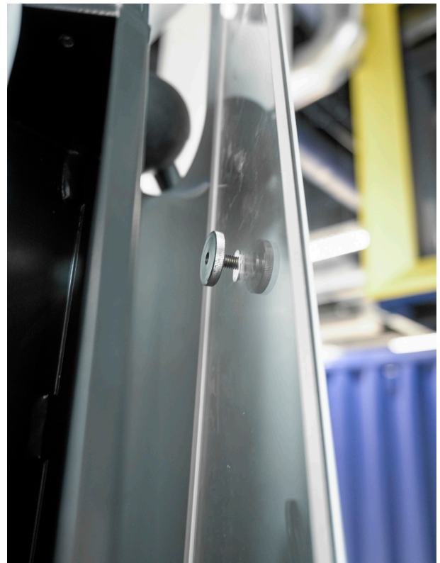
Figure 27. Furthermore, to remove the side panels 8 thumb screws have to be unfastened. Another low visibility penalty is given here.
