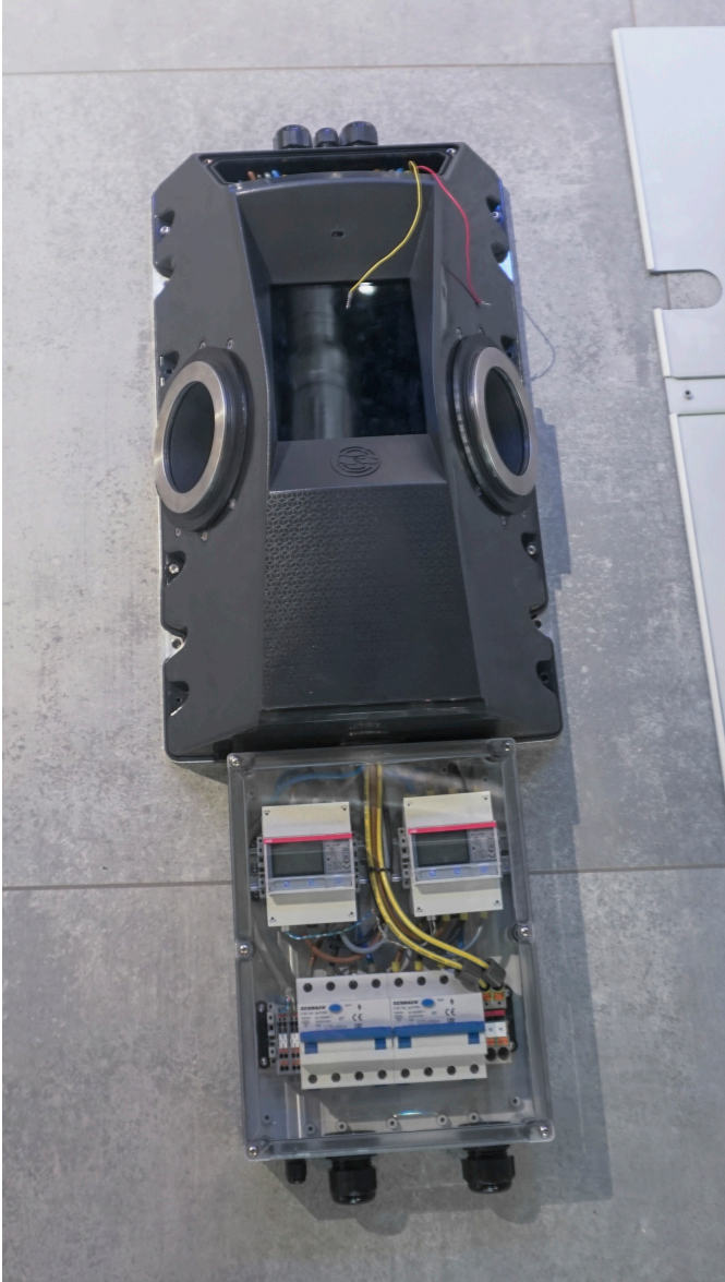
◀ Figure 30. The charger- and installerbox are handled as one rigid unit. They are connected with a cable tree and a threaded connection which is part of the aluminium chargerbox heatsink/ backplate.
