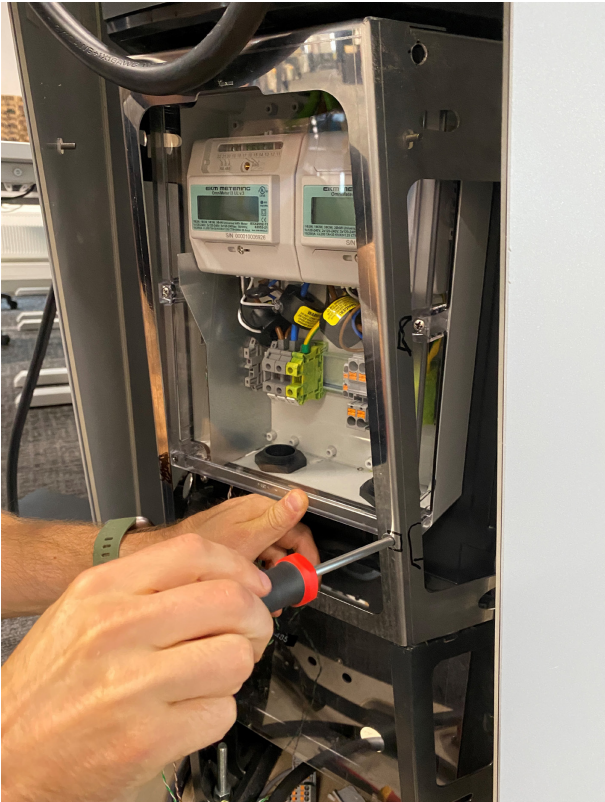
▲ Figure 71. The screws are accessible with the addition of 6 holes in the bracket. There is not enough space to remove the lid, however.
