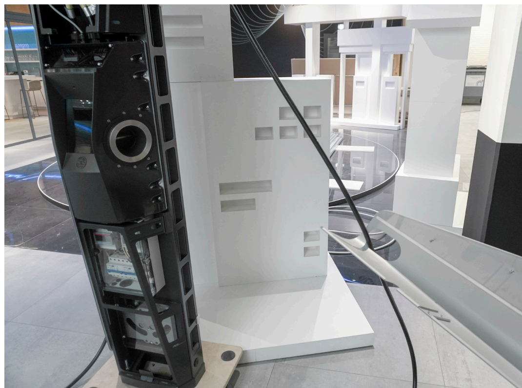
Figure 29. Removal of the side panels means manoeuvring them over the charger cables.
