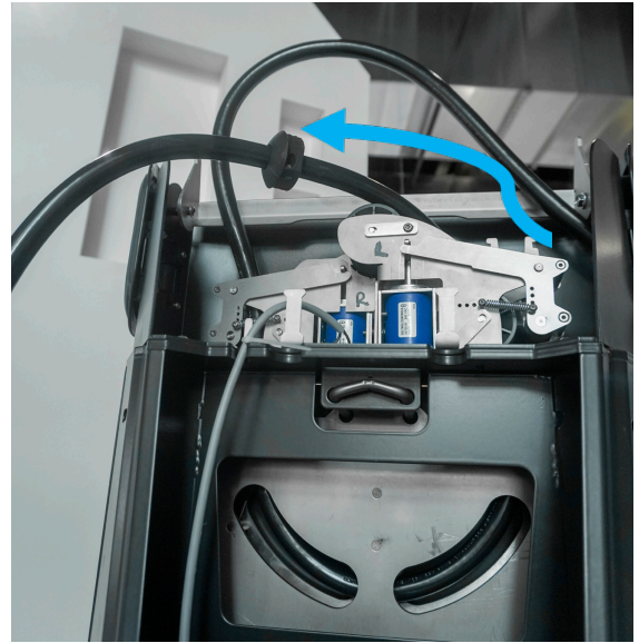
▶ ▲ Figure 75 & 76. The stoppers need to be pulled out of the product and towards the de-installer to be disassembled.
