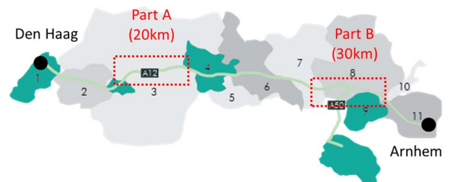
Fig. 17. A12 highway between Den Haag and Arnhem with IPT system installed over two section – Part A for 20 km and Part B for 30 km.
