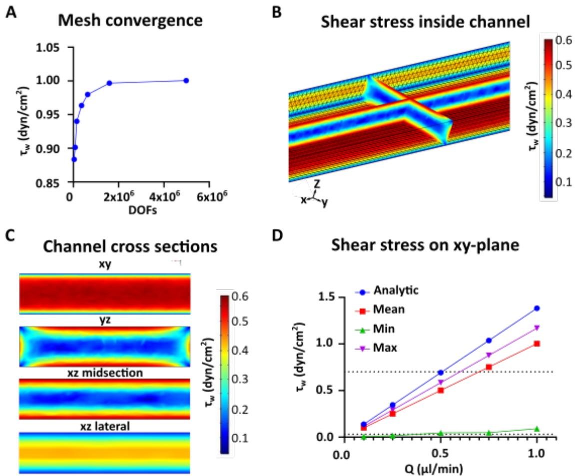
Figure 3.7: **A)** The change of the mean wall shear stress,  $\tau_w$ , using different mesh sizes, DOFs. **B)** Wall shear stress,  $\tau_w$ , in the middle of the channel. **C)** Wall shear stress,  $\tau_w$ , of 4 different cross sections of the channel. **D)** The analytical calculated, mean, minimum and maximum wall shear stress,  $\tau_w$ , induced on the bottom of the channel at different flow rates  $Q$ .
