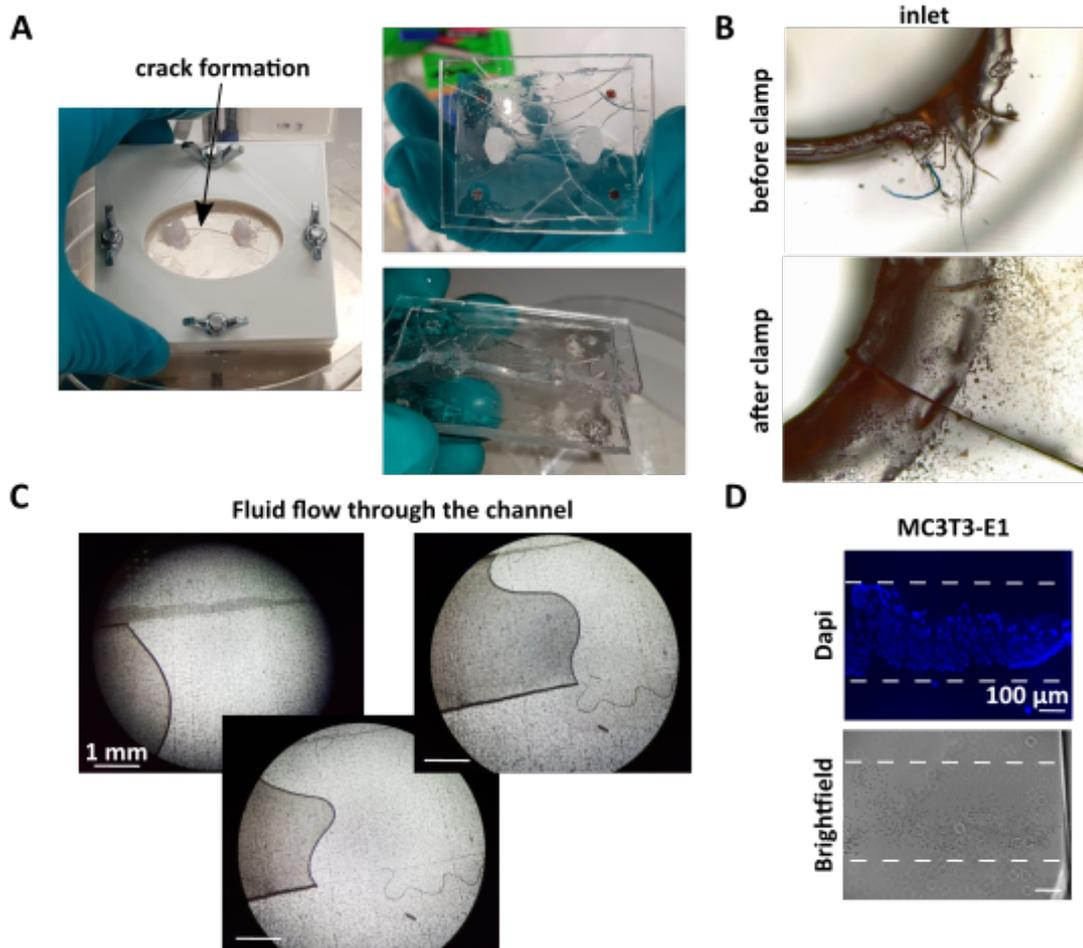
Figure 3.11: **A)** Crack formation around the inlets of the dynamic chip. **B)** Closer look at the crack formation before and after usage of a clamp, images were taken with the LEICA DM 590. **C)** Fluid flow through the channel inside the chip images were taken with the LEICA DM 590. **D)** Dapi staining of the waver, after MC3T3-E1 cell seeding inside the dynamic chip.
