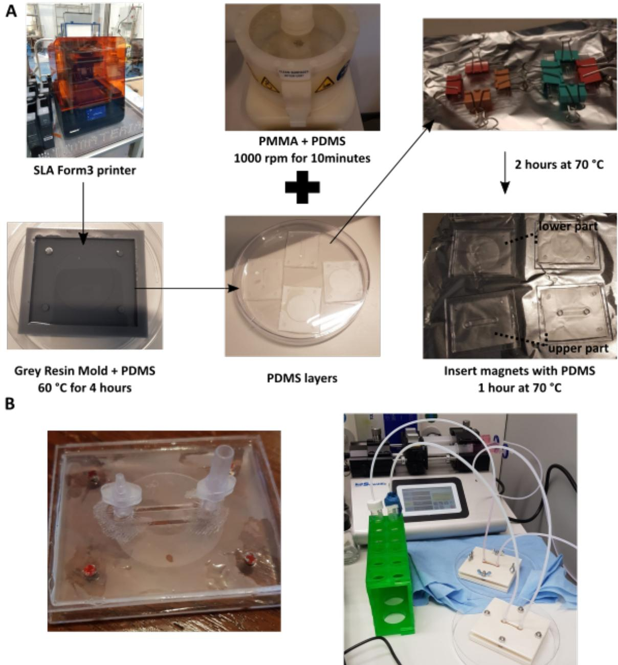
Figure 3.10: **A)** Microfluidic chip fabrication steps **B)** (left) Final chip design with two different luer connectors. (right) Two microfluidic chips attached to the Legato 270 syringe pump
