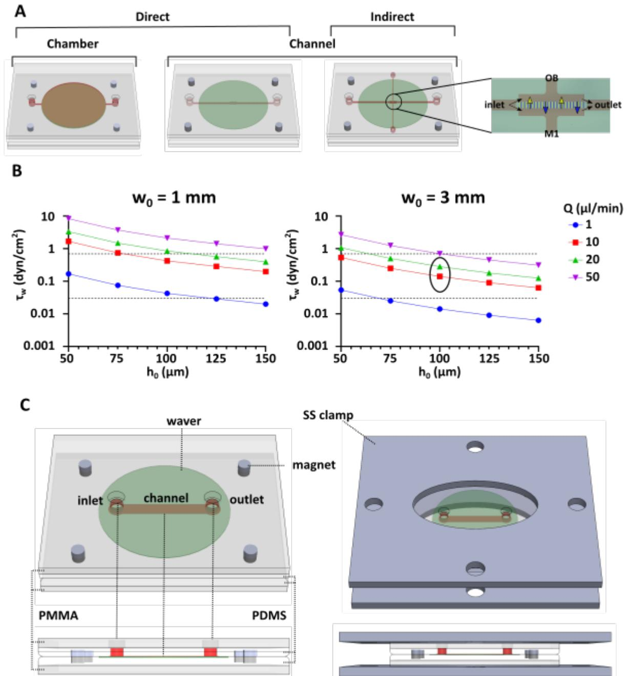
Figure 3.9: **A)** Initial microfluidic chip designs **B)** The resulting mean Wall shear stress,  $\tau_w$  at different flow rates,  $Q$ , in  $w_0 = 1\text{ mm}$  and  $w_0 = 3\text{ mm}$  rectangular channels with different heights,  $h_0$ . **C)** Final design without and with clamp
