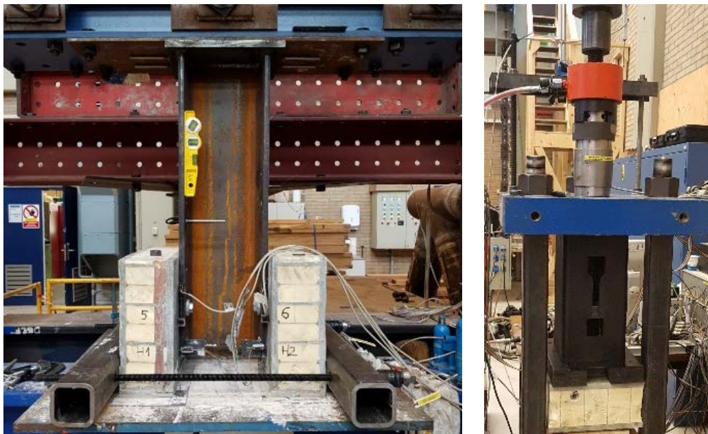
Figure 1. Push-out (left) and pull-out (right) tests
