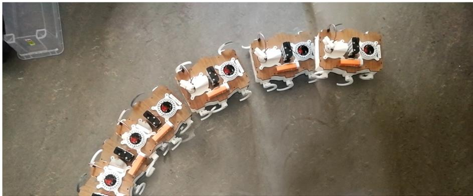
**Figure 6-2:** Example of the turning of the ZeBRo using Max-Plus based turning
