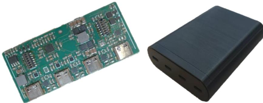
Figure 12: PCB of a power-bank prototype and its 3D printed case
