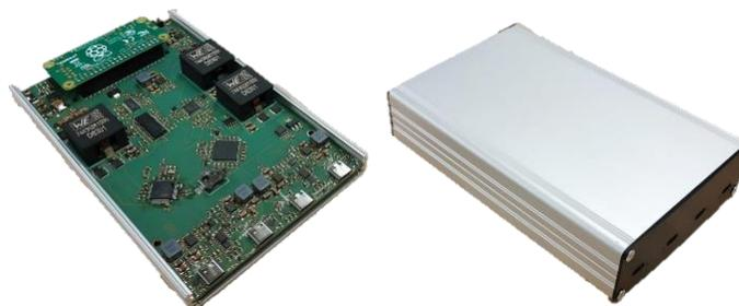
Figure 11: PCB of a solar charging station prototype and its case
