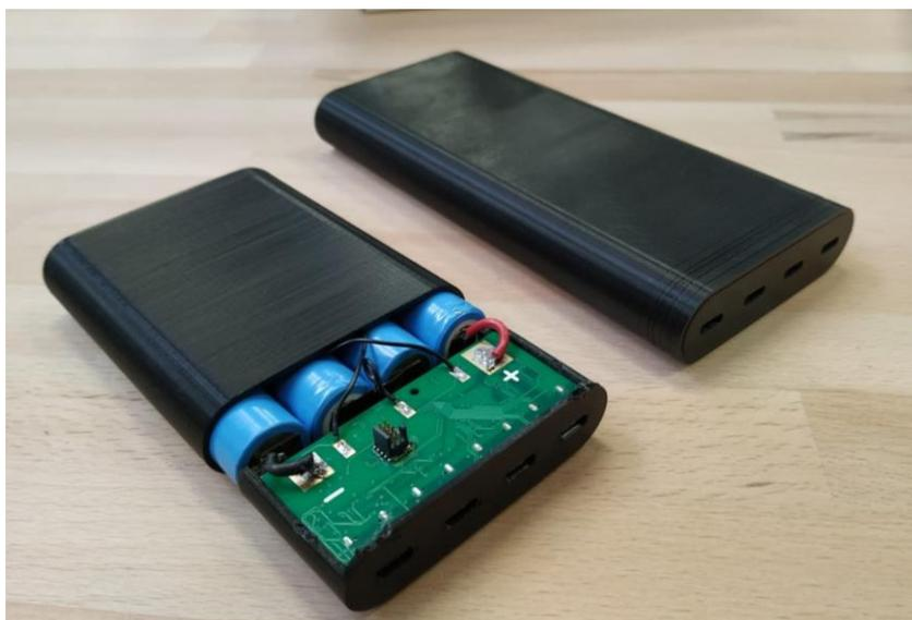
**Figure 49: A 4-cell power-bank prototype on the left and an 8-cell prototype on the right**
