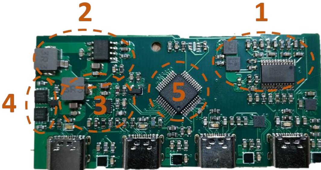
**Figure 47: Prototype of the power-bank second revision with highlighted elements**
