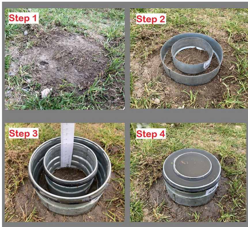
Figure 75: The placement and use of the double ring infiltrometer
