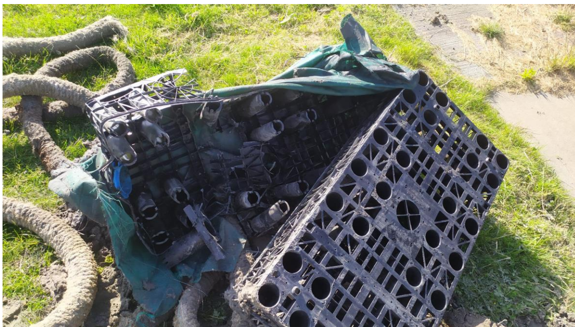
Figure 83: Infiltration box and drain.
