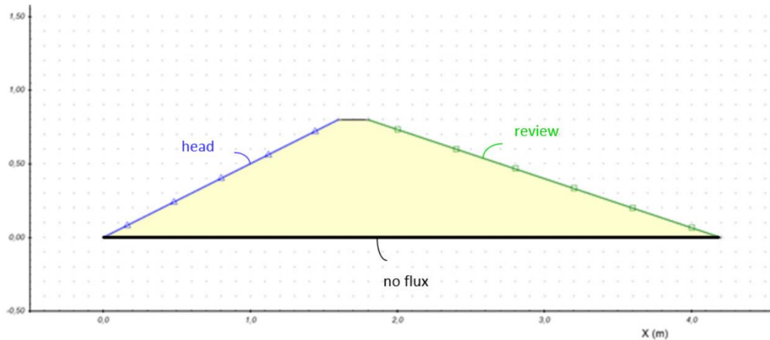
Figure 26: Boundary conditions for numerical model of WaterLab reference case
