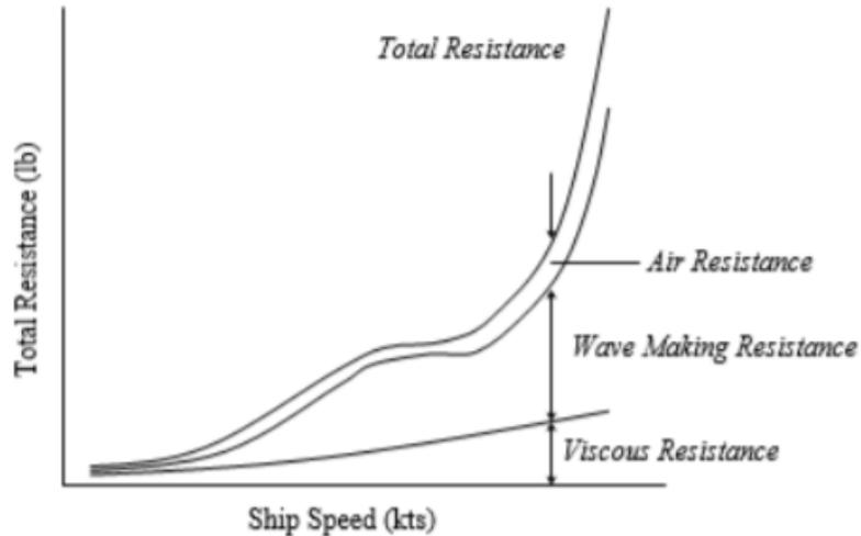
**Figure 1.10:** Components of hull resistance with varying speed [130]
