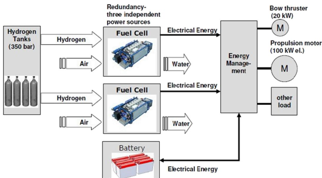
Figure 2.4: Generalized hydrogen power plant system [126]
