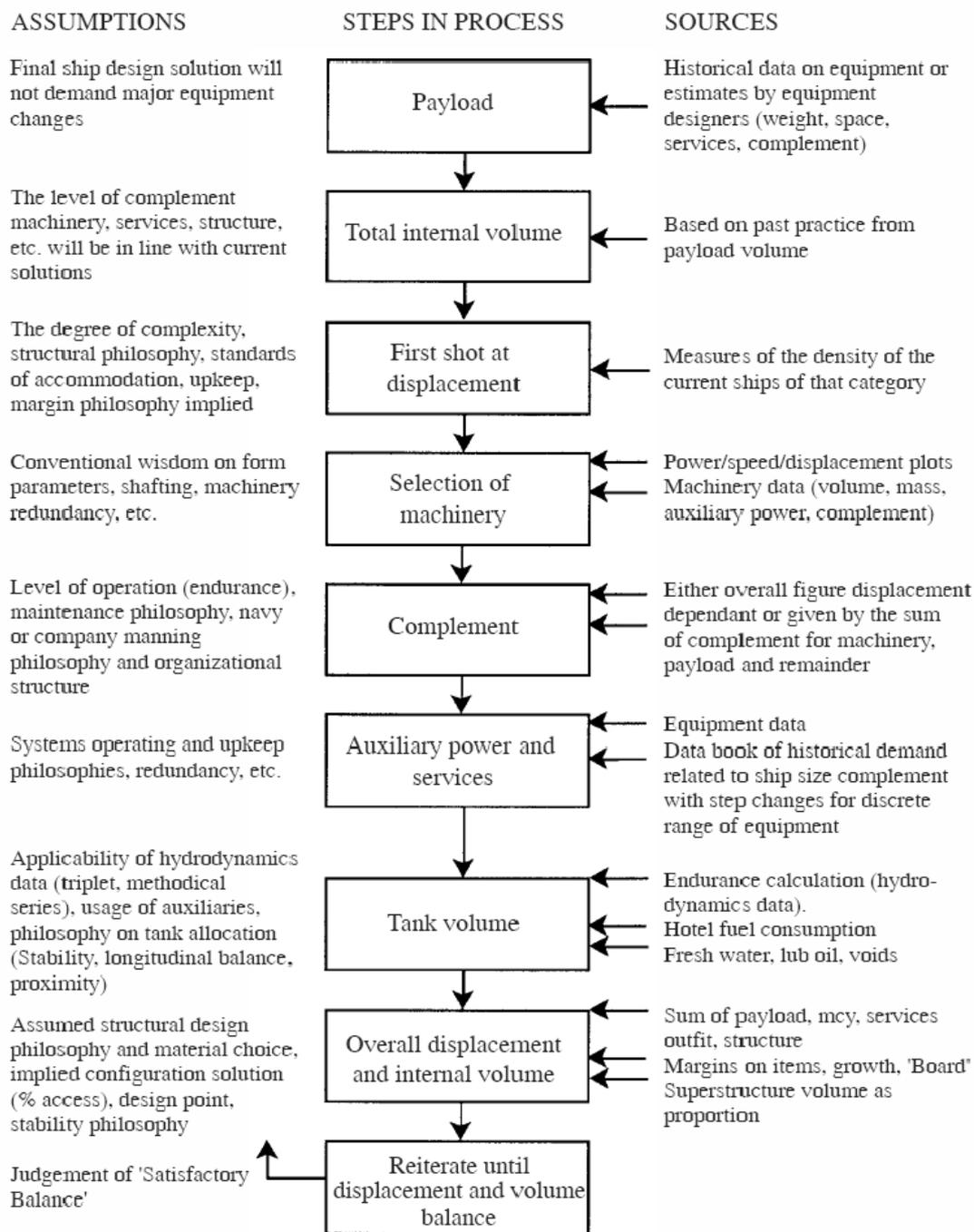
Figure 1.9: A simple numeric ship sizing iterative sequence with feedback [7]
