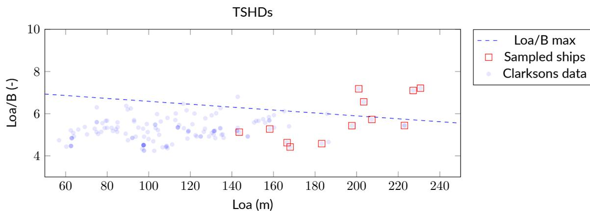
Figure 2.10: Length-beam ratio of Clarksons data and sampled TSHD
