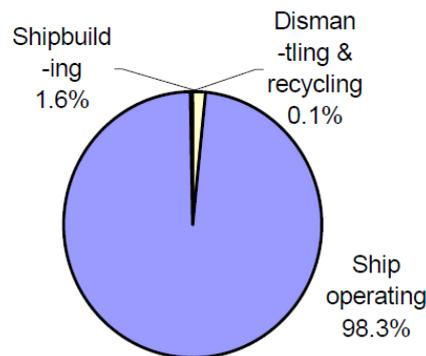
Figure 1.5: Panamax bulker environmental impact share per stage [77]
