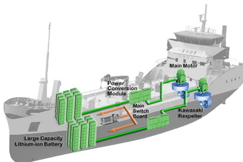
Figure 2.6: Generalized Li-ion battery power plant system [78]
