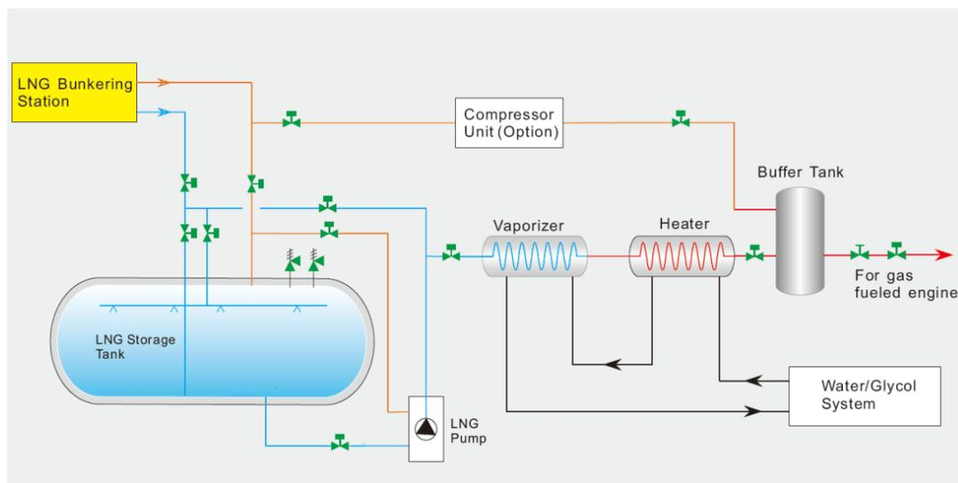
Figure 2.3: Partial generalized LNG power plant system [86]
