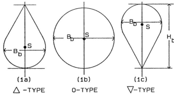
Figure 3.3: Typical bulbous bow transverse shapes [2]
