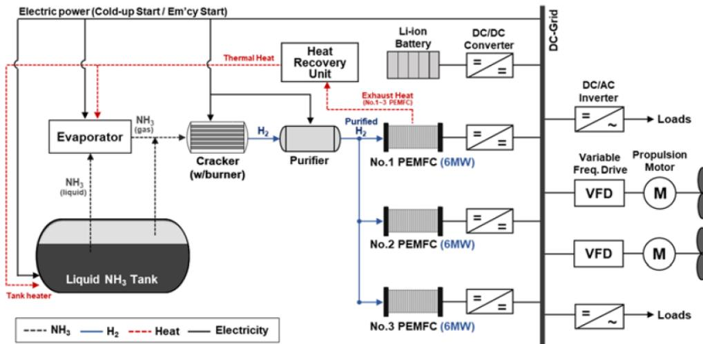
Figure 2.5: Generalized ammonia power plant system [79]
