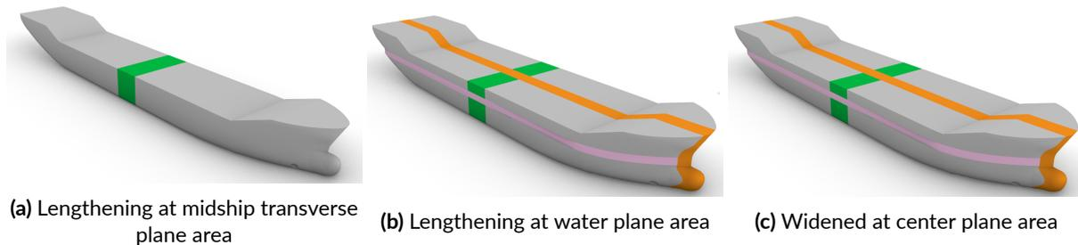
**Figure 3.5:** The design generation sequence to accommodate additional AMEC bunker space
