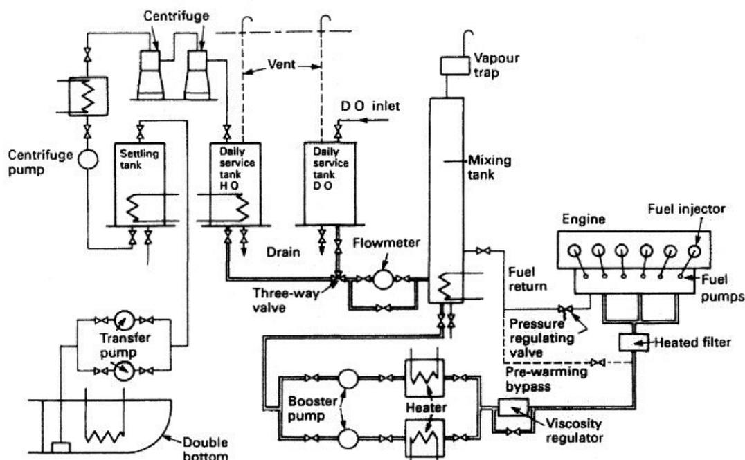
Figure 2.1: Generalized fuel oil power plant system [93]
