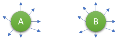
Figure 5.1: In the "broadcast dissemination" solution, the nodes performing a transaction disseminate the its information to the entire network.
