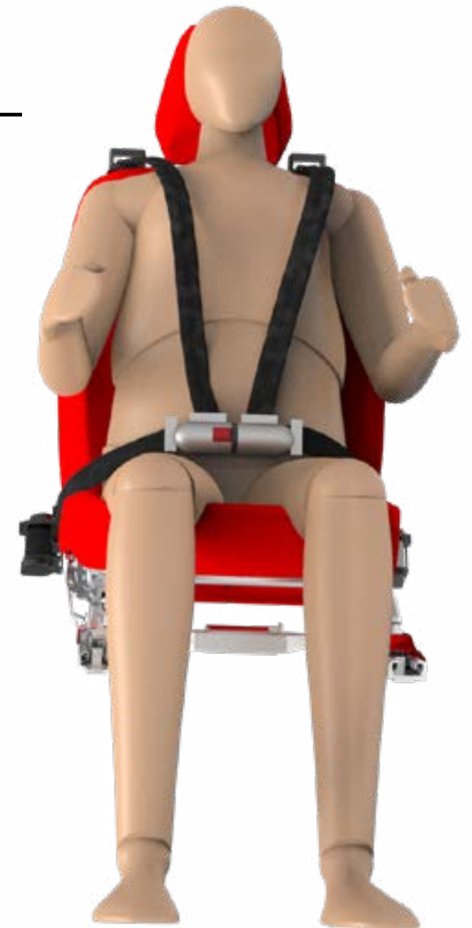
Fig 63 : Four point configuration in a reclined position.
