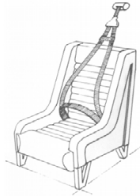
Figure 12: Y- yoke integrated system by H McElhaney,(1972)
