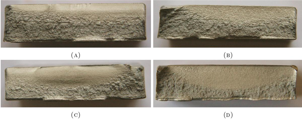
FIGURE 3.24: *Fracture surfaces of test specimen. (A) failure at corner,  $S = 220$  [MPa], (B) failure at undercut,  $S = 220$  [MPa], (C) failure at corner,  $S = 140$  [MPa], and (D) failure at undercut,  $S = 140$  [MPa].*
