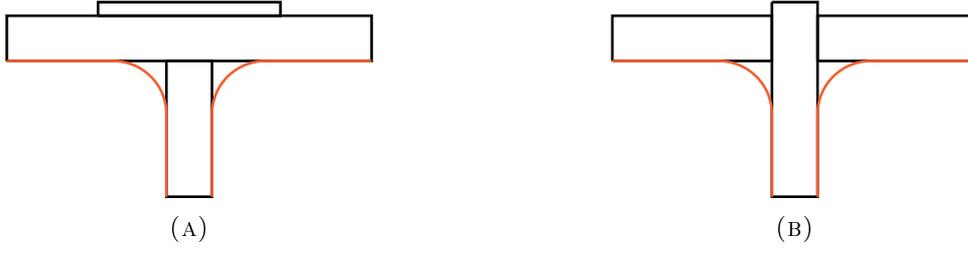
FIGURE C.9: Schematic view of DS T-lap-joint (A) and DS T-butt-joint (B) used as structural details in the fatigue analysis of de Jesus et al. [21]. The red lines represent the mould.
