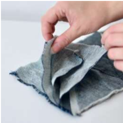
Figure 3: Sample of a 3D woven denim structure.
