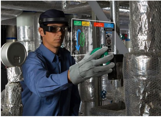
Figure A.7: Composite image of AR application with partial spatial-mapping. [14] The worker in the scene is using a pair of Epson Moverio BT-200 to access virtual content related to the real object in front of him but not conformally overlaid to it [14].
