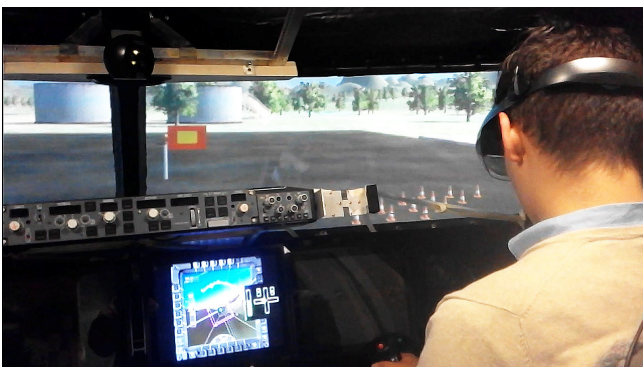
Figure 10. Prototype setup with participant wearing the AR goggles. The picture was taken after the end of the experiment and features the cockpit illumination that would normally be maintained off. Also note that information on the instrumentation panel is fixed and not relevant for the experiment.
