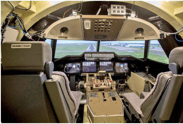
Figure 2. Cockpit of the SRS in typical fixed-wing configuration, with yoke on the left seat and side-stick on the right seat (Ref. 14).
