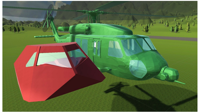
Figure 3. Cockpit 3D models for the (left) and the S-70 (right), with the two models shaded in different colors and separated horizontally for illustration purposes. In the simulation the two models coincide, with windows completely transparent and the cockpits in a black unlit material with no reflective properties (occlusion mask).
