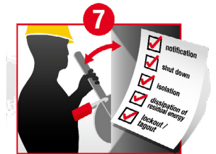
Inspection of isolation 1 & 2
