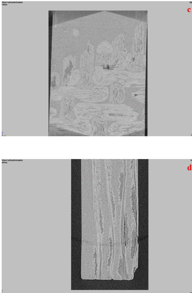
Figure 5.9 Tomographic images of the Carbon-fiber composite. a: top down view about 0.2 mm below the surface showing large scale delamination, an almost pure polymer layer and some small scale delaminations, b: 2 nd view of the delaminated region at another viewing plane, c: top down view at another location and d: cross-sectional view.
