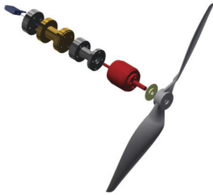
Fig. 2. Exploded view of the propeller drivetrain.
