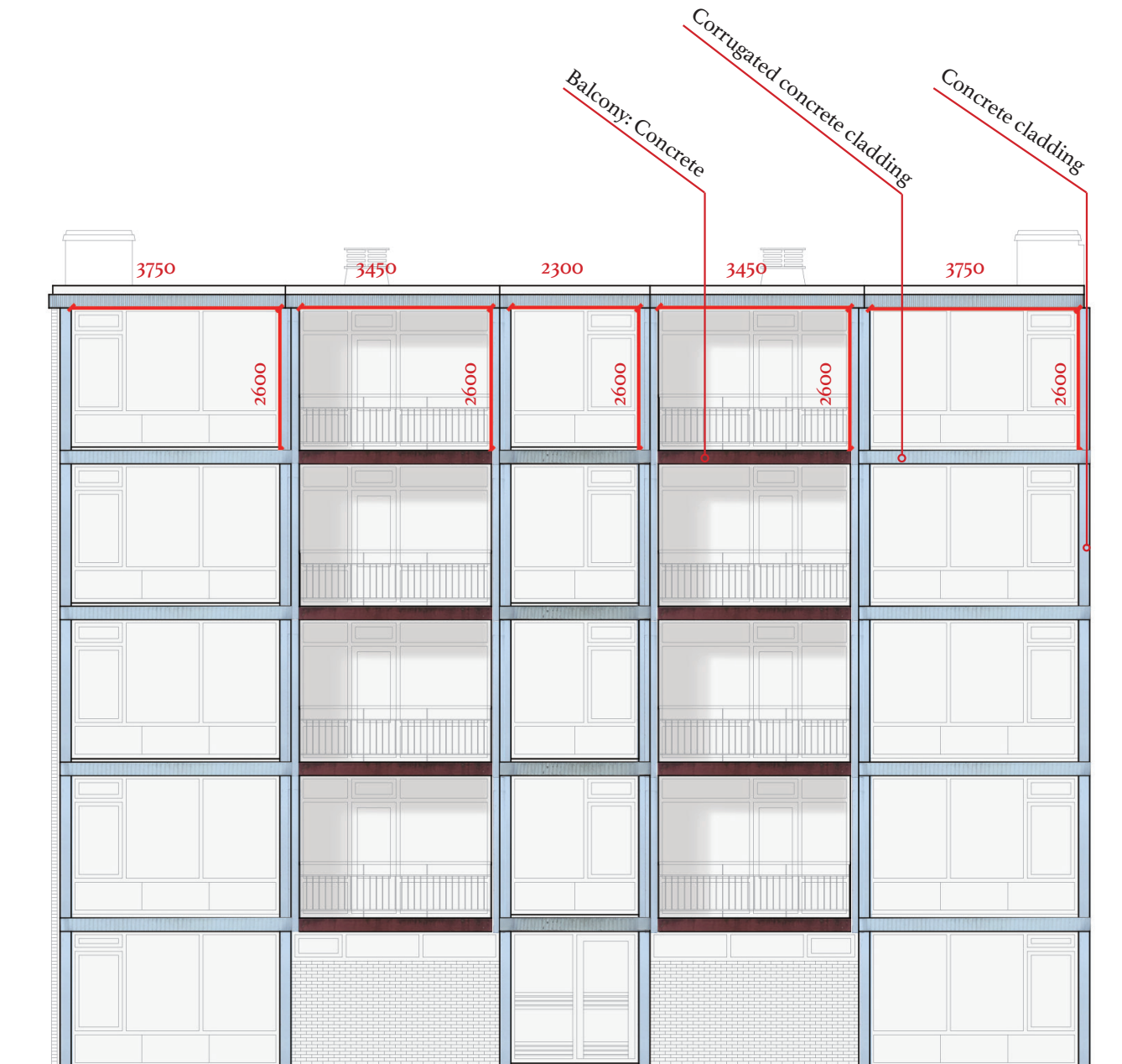
Figure 1.3.3 Overview of Concrete Frame in one portiek
