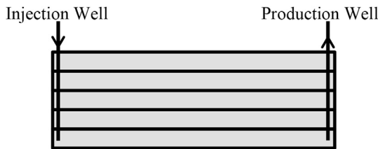
Fig. 2. The case study: a five-layer rectangular reservoir with one producer and one injector.
