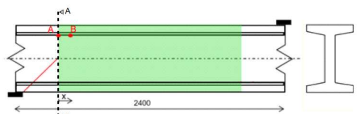
Figure 7-35 Location of maximum principle stresses (LB6)
