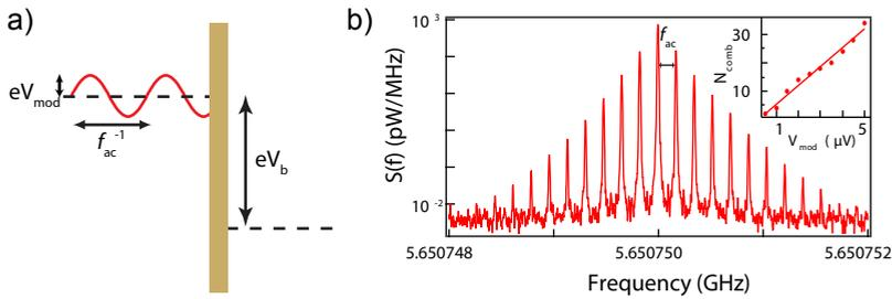
Figure 5.12: Frequency comb generation. **a) – b)** Low frequency ( $f_{ac} = 111\text{Hz}$ ) modulation of the voltage bias across the SQUID under injection locking conditions generates a frequency comb of phase coherent signals spaced  $f_{ac}$  in frequency around the center emission frequency. (Inset) The comb width,  $N_{comb}$ , is controlled by  $V_{mod}$ , the amplitude of the modulation on the voltage bias.
