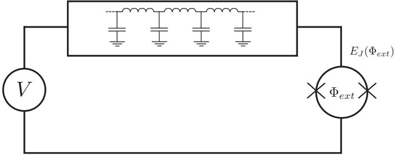
Figure 5.13: Circuit schematic. Circuit diagram of a voltage-biased Josephson junction in series with a resonator. The Josephson energy of the junction  $E_J(\Phi_{ext})$  can be tuned by an external magnetic flux  $\Phi_{ext}$ .
