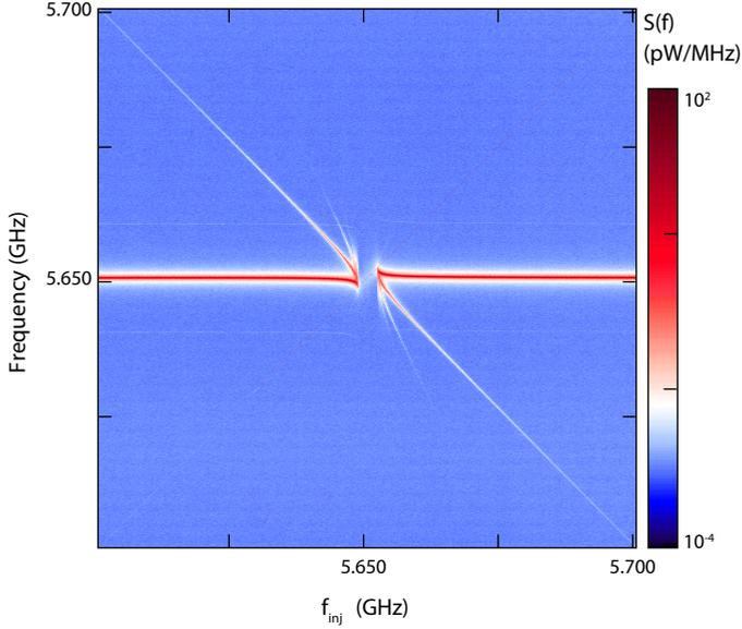
Figure 5.10: Injection locking - Sideband range. Power spectral density  $S(f)$  as a function of frequency of the injected tone for an input power  $P_{inj} = -90\text{dBm}$  showing creation of sidebands spanning more than 100MHz.
