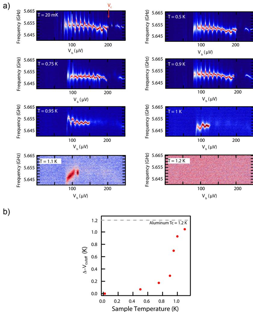
Figure 5.9: Temperature dependence of the emission. **a)** Power spectral density  $S(f)$  of the emission as a function of voltage bias for different sample temperatures. **b)** The emission cutoff point  $V_c$  scales strongly with temperature close to the superconducting critical temperature of Aluminium, indicating that the upper cutoff of the emission  $V_c$  is set by excitation of quasiparticles that damp the junction.
