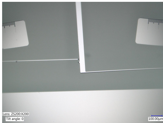
(a) Broken beam
