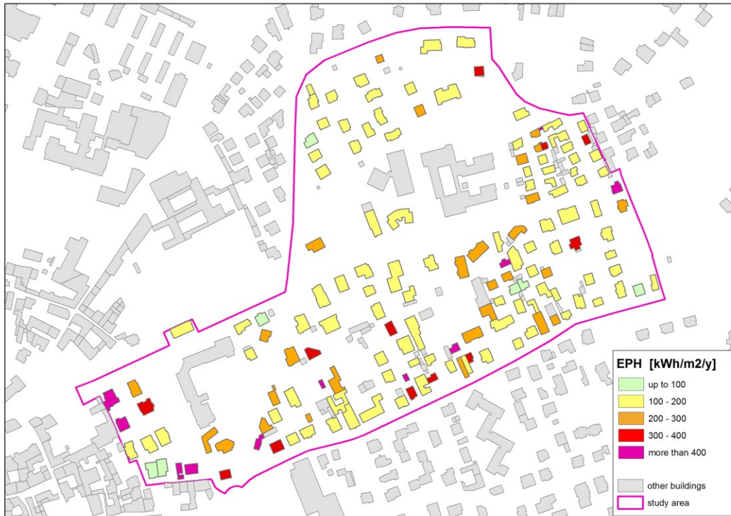
Figure 14. Estimated energy consumption for the retrofitting scenario “Windows improvement”. Image source: authors.
