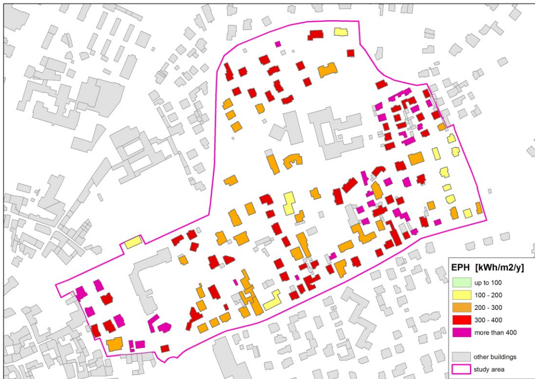
Figure 7. Heating energy demand computed with data package DP1. Image source: authors.
