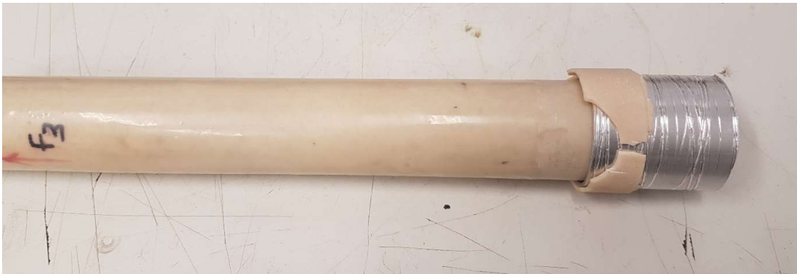
Figure E.6: Core to be stacked with guiding aluminium tube
