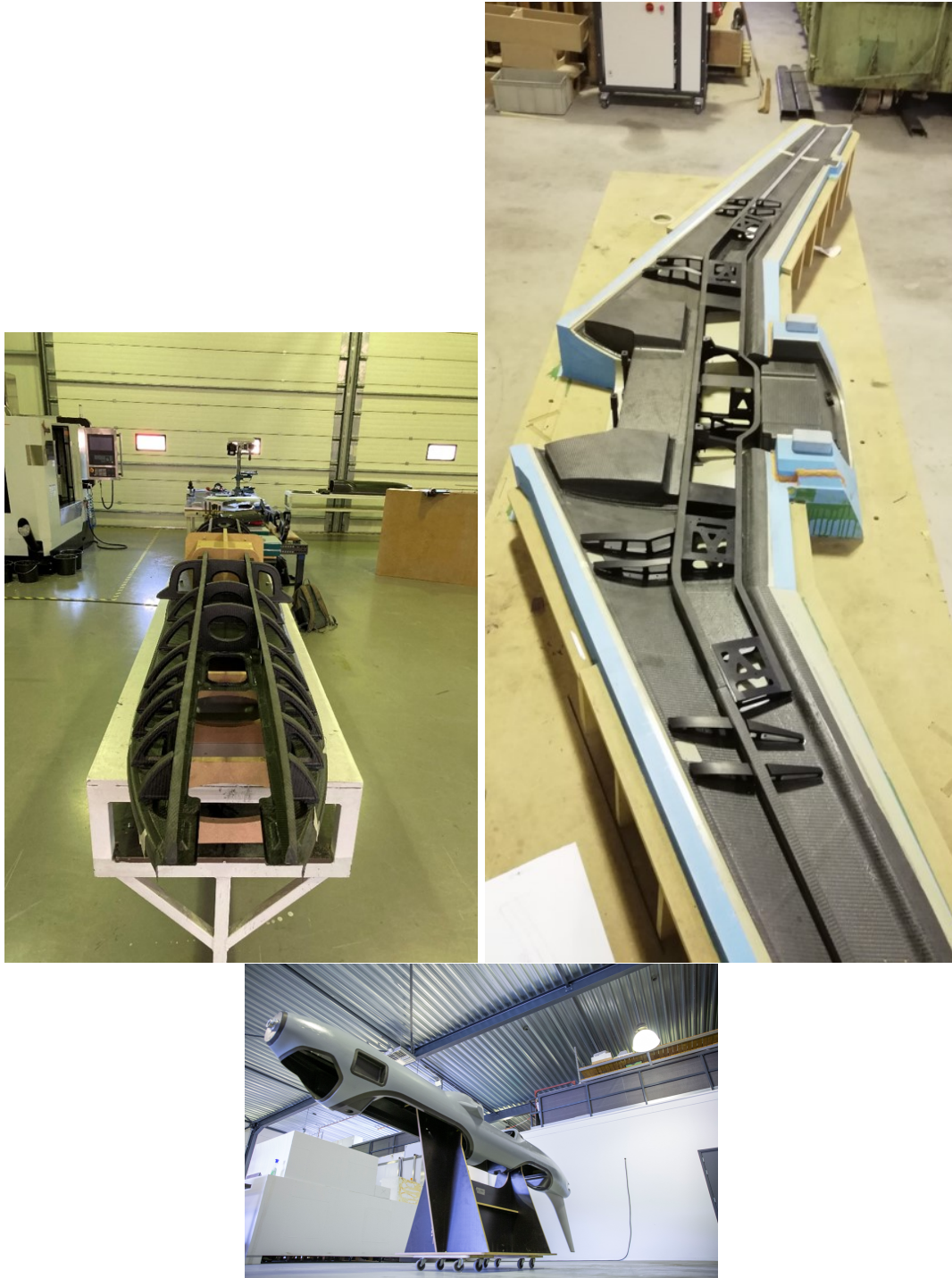
Figure 6. Structural parts of the fuselage and the assembly of the wing and the fuselage.
