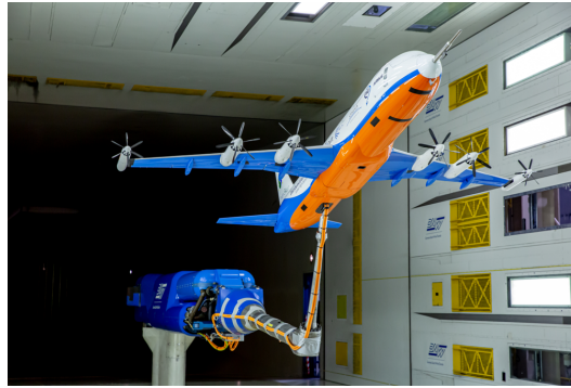
Figure 7. The DEP-SFD D08 in the DNW windtunnel facilities in Marknesse, The Netherlands.
