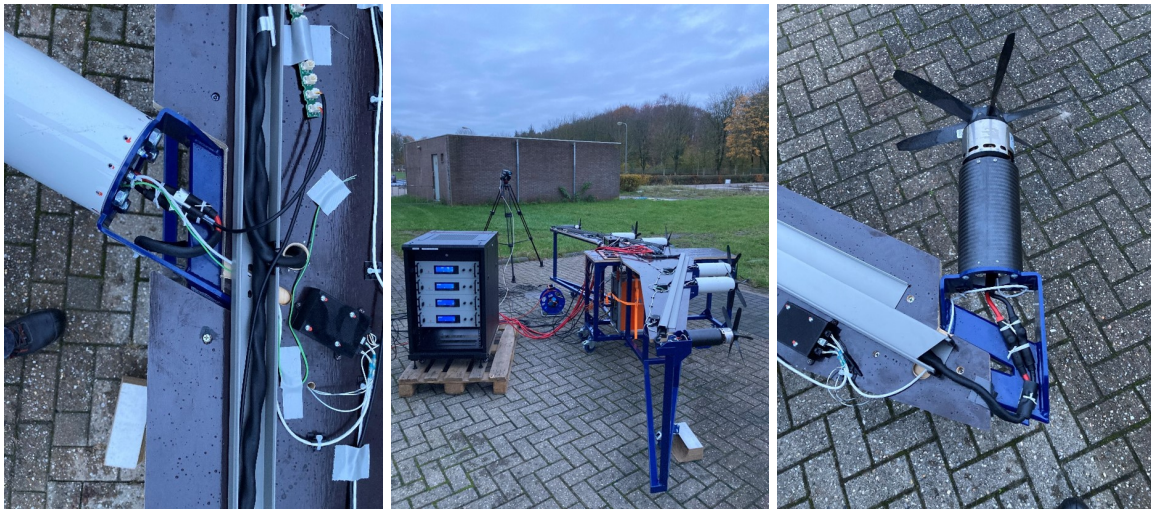
Figure 14. The iron-bird of the DEP-SFD2.
