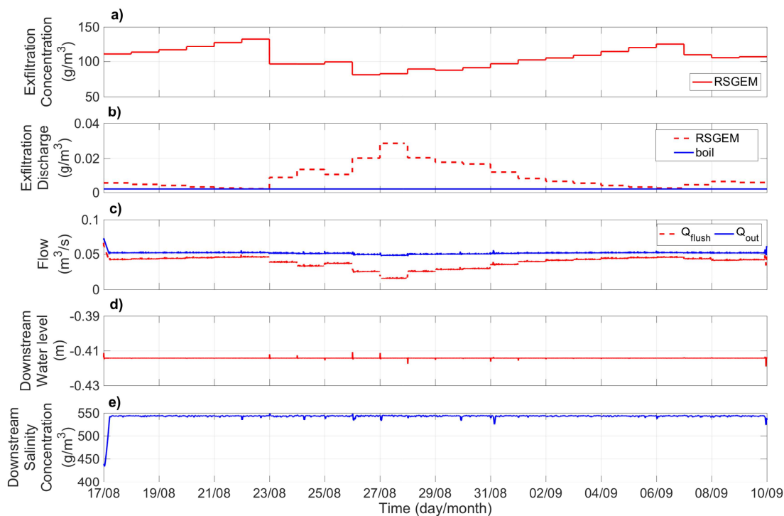
Figure 5 Disturbance data and results of the controller for the first scenario. Groundwater exfiltration a) concentration ( c_{\text{boil}}=5453 \text{ g/m}^3 is constant and not shown in the figure) and b) discharge used for the first scenario (dashed lines shows the first location 40 m downstream of the flushing inlet which is a combination of the first boil and the exfiltration modelled by RSGEM and the solid line shows the second location which is 60 m downstream of the flushing inlet with the second boil only). c) Controlled flushing and outflow discharge, d) downstream water level and e) downstream salinity concentration.
