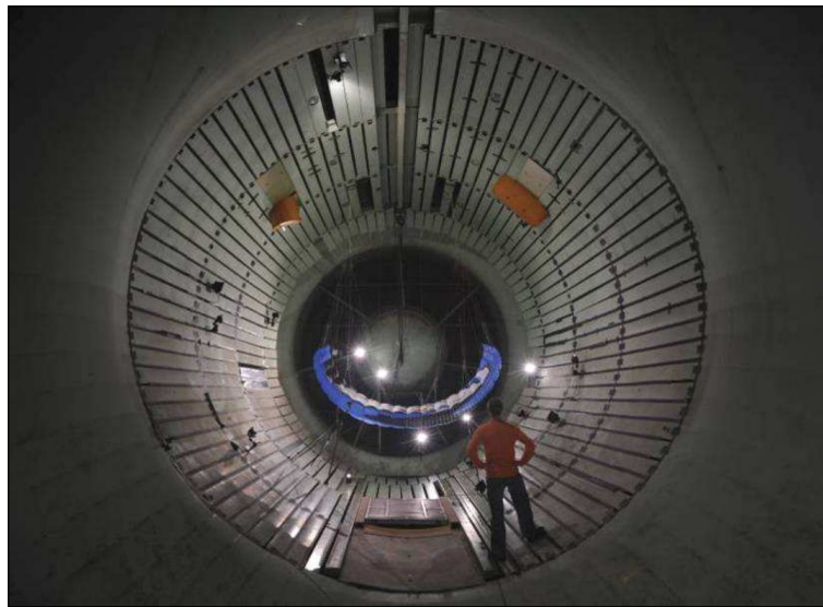
Figure 2.23: Ram-air kite during wind tunnel test [74].
