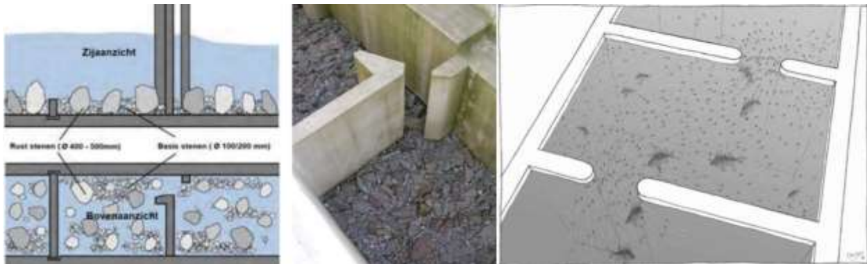
Figure 42: The advised 20 cm thick substrate layer for fish passages (Ghodrati, 2021)[left] and the Meandering flow pattern of the fish passage (Coenen, Antheunisse, Beekman, & Beers)
