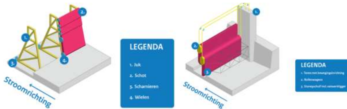
Figure 62: Main components of the combined Poirée and Stoney weir (Ankum, Delbressine, Kurvers, & Maes, 2023)
