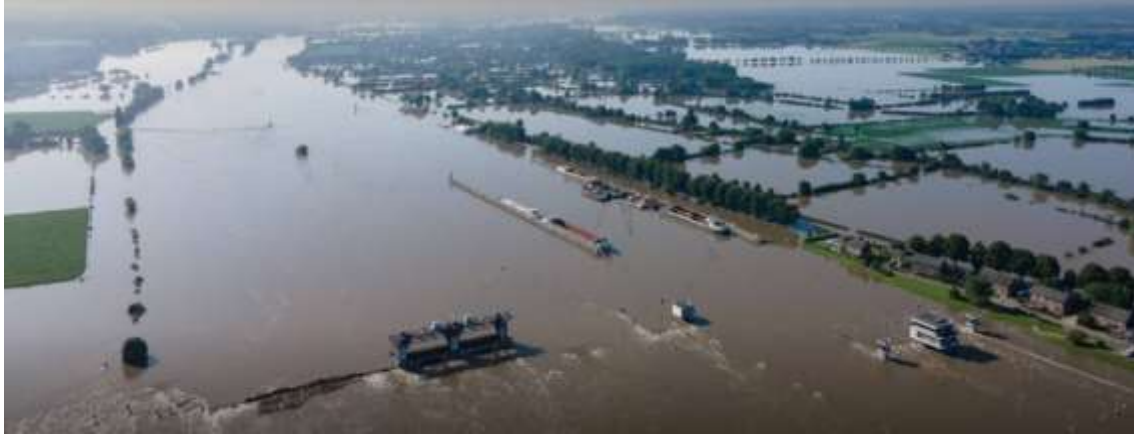
Figure 14: Floodplains surrounding weir complex Sambeek during flood river discharges ( Q_{river} > 1600 \text{ m}^3/\text{s} ). This image was taken during the floods of 2021, which was an exceptional situation (Heijligers).
