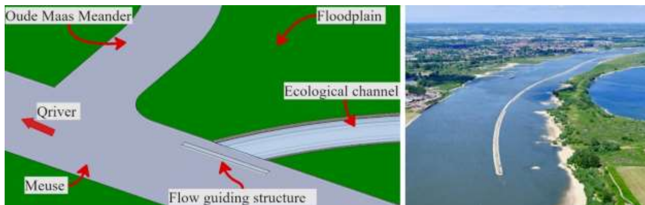
Figure 30: The figure on the left gives an impression of the flow guiding structure at the channel's outlet (it is not drawn to scale). The figure on the right shows a longitudinal dam on which the flow guiding structure is based (Siebe Swart, 2020)
