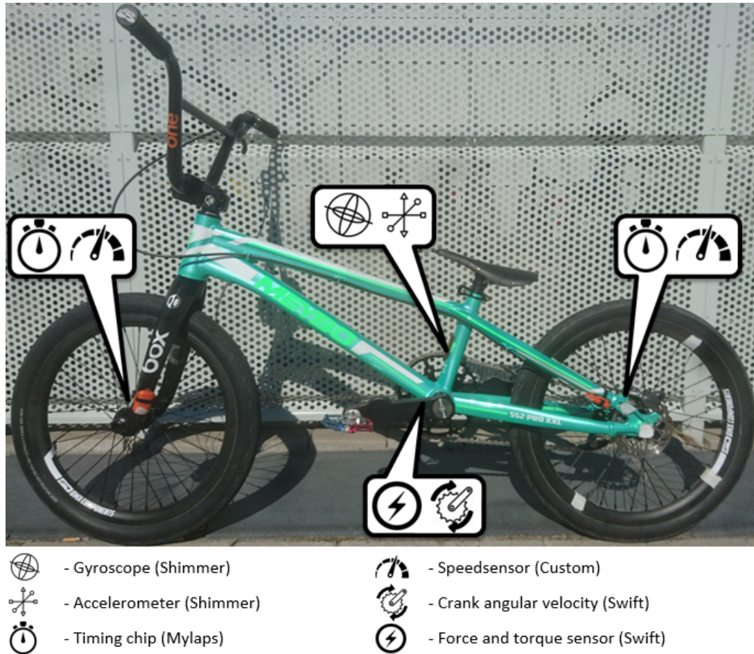
Figure 2.2: The instrumented BMX bicycle (Holeshoot, Meyboy, Boxmeer, Netherlands) equipped with multiple sensors. Additionally white tapes on the rear rim every 90^\circ make rear wheel rotation better visible on the video recordings.
