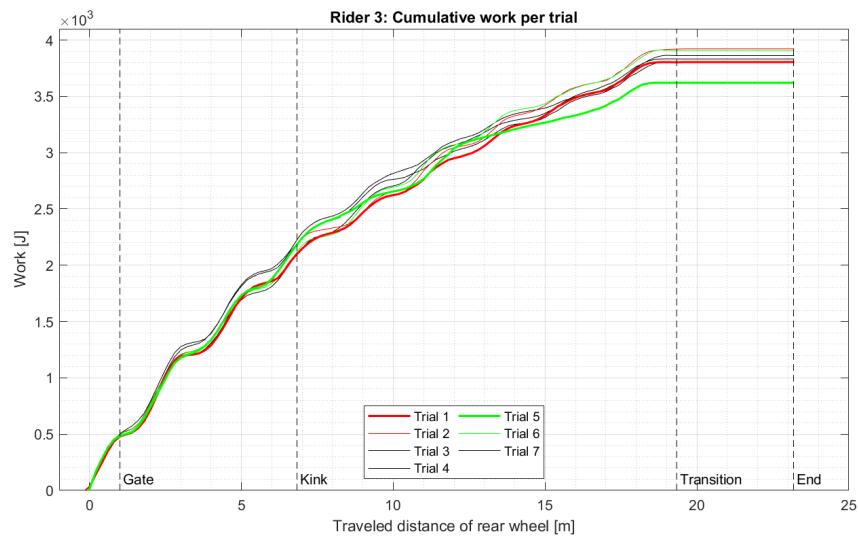
Figure C.3: Cumulative work done by rider 3 for every trial over the traveled distance on the start ramp. In red (Trial 1 and 2) the two slowest start times ( t_{end} ) in which the bold line is the slowest trial (Trial 1), in green (Trial 5 and 6) the two fastest start times in which the bold line is the fastest trail (Trial 5). The horizontal line at end of the ramp means no added work over that distance, i.e. stopped pedaling at the end of the ramp to prepare for jump.
