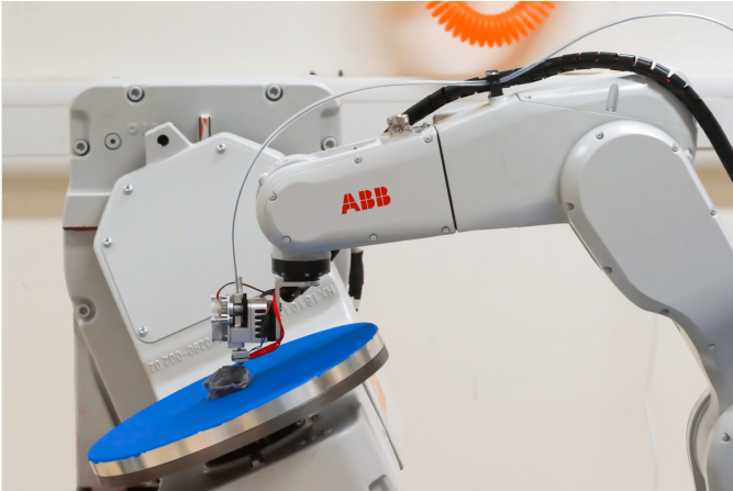
Fig. 8. A hardware setup of robot-assisted 3D printing system with 8-DOFs consisting of a 6-DOF ABB IRB1200-7/0.7 robotic arm and a 2-DOF IRBP A-250 tilting table.
