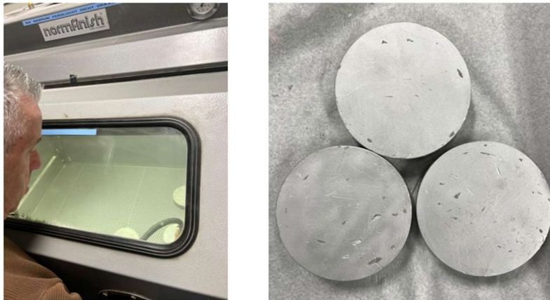
Figure B.13. Sandblasting process and sandblasted loading platens.
