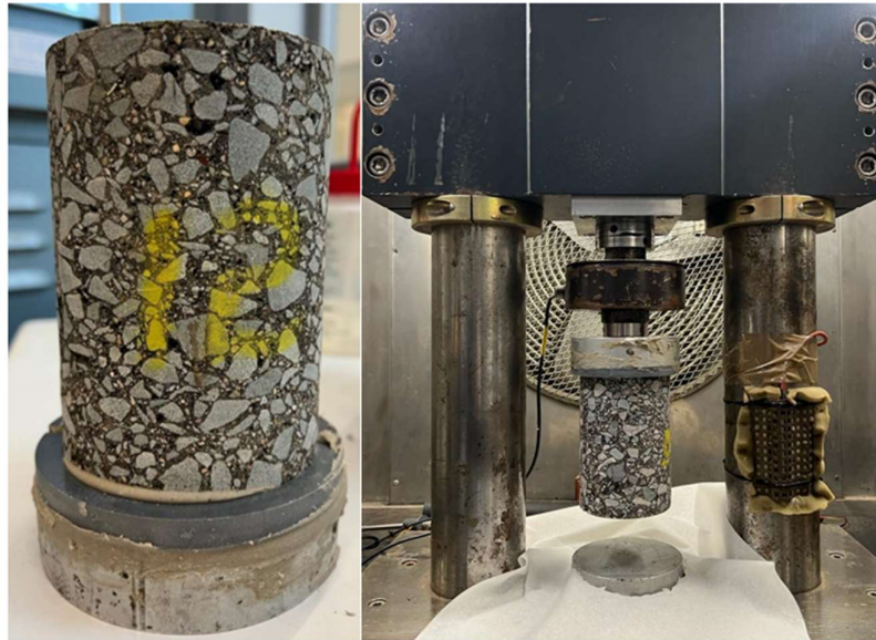
Figure 4.6. Gluing (a) the lower end of the specimen and (b) the upper end under compression loading.
