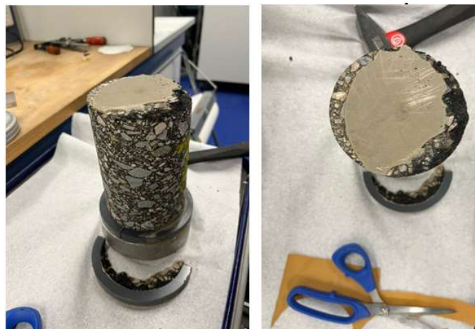
Figure B.3. Failure in asphalt material while removing the glue.
