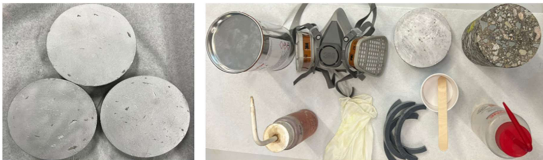
Figure 4.5. (a) Sandblasted loading plates and (b) different equipment required for end treatment (Powdered glue, 3M mask, specimen, hardener, rubber gloves, PVC rings, Mixing cup & Acetone).
