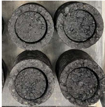
Figure B.10. Cores and shell for gyratory compacted specimen.
