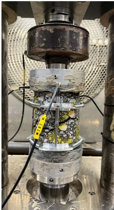
Figure 2.12. Test setup for uniaxial fatigue and healing testing.
