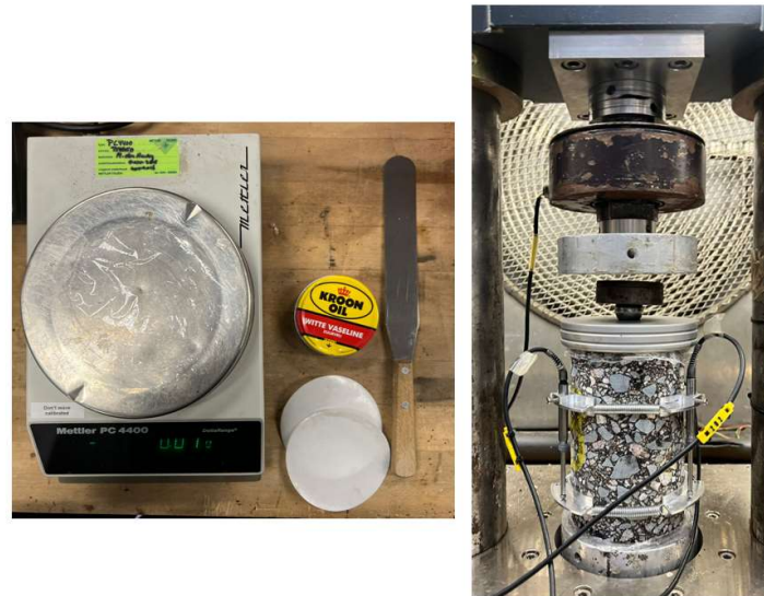
Figure 4.4. (a) White Vaseline and plastic sheet for end treatments (b) Ball and plate arrangement for uniform load distribution in stiffness testing.
