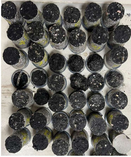
Figure B.15. Failed specimens after fatigue & healing testing.
