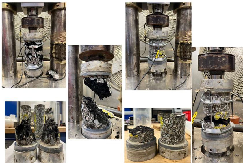
Figure B.9. Failure pattern in the tension-compression mode of loading.
