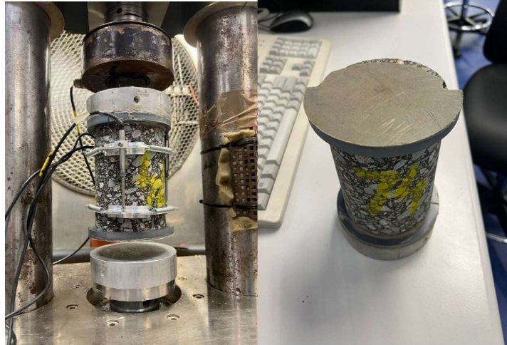
Figure B.2. (a) Glue line failure in specimen during fatigue testing and (b) intact specimen along with glue.
