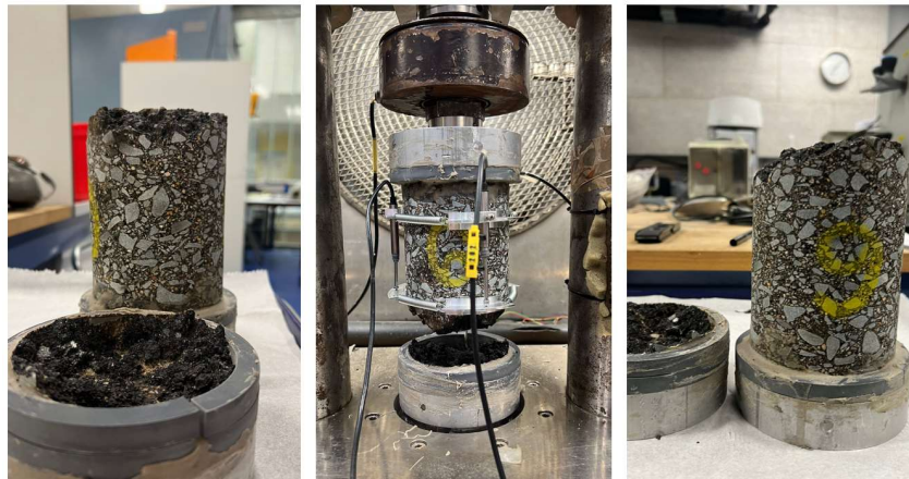
Figure B.6. Failure pattern in pure tension mode of loading.
