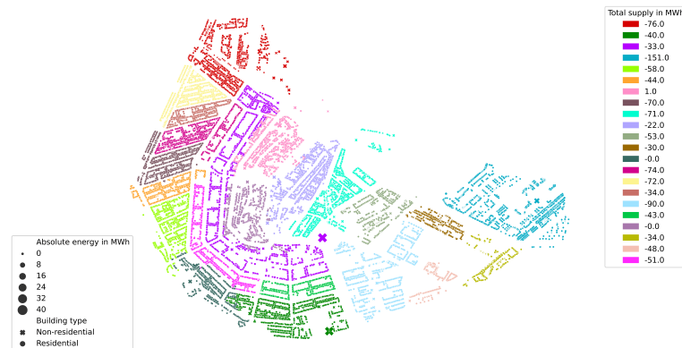
Figure 5.5: Clustering the inner city of Amsterdam, coldest day
