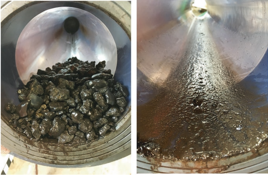
Fig. 4.11 The nodule batch after the experiments (left), the developed fines due to degradation (right). (From: de Hoog et al., 2020. Copyright Elsevier 2020, reprinted with permission)
